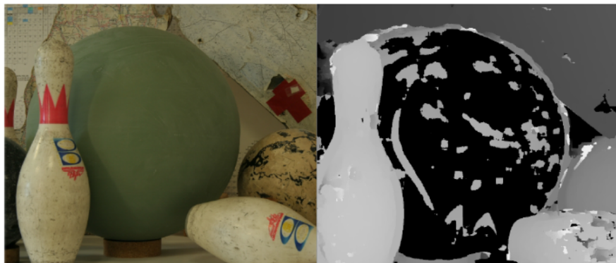
Figure 10: Disparity map using block matching technique
