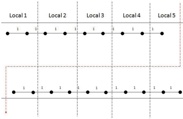
Fig. 12. Suppose the detection gain threshold is 1. Even all pairs of neighboring local regions ensure barrier coverage for their merged region, there still exists a crossing path with detection gain 0 as the arrow line.
