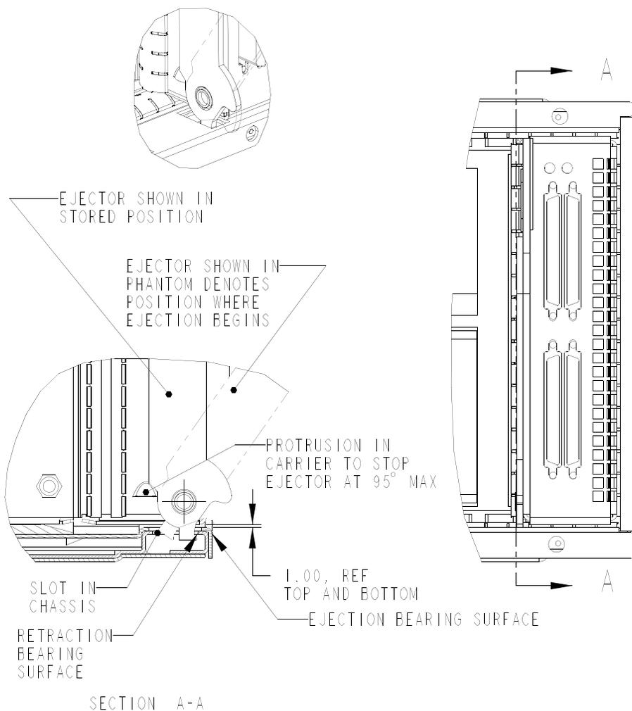
Figure 118 Chassis slot/Ejector Interface
