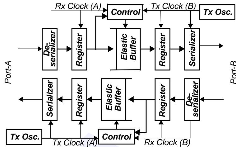
Figure 29 A Conceptual Retiming Repeater Block Diagram
