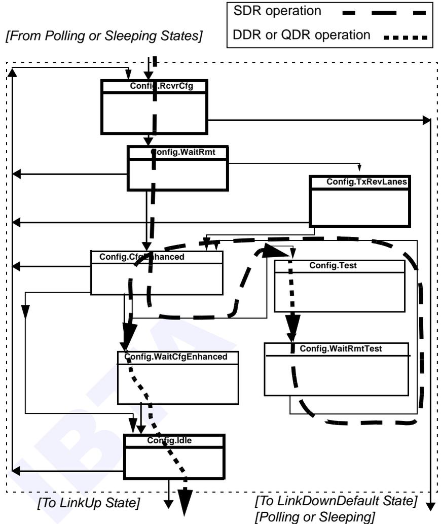
Figure 27 Typical Control Flow through Configuration Super State - Enhanced Signaling
