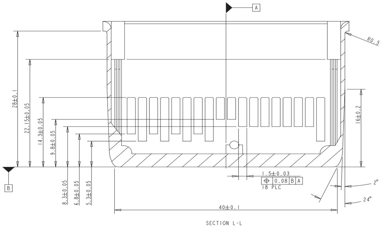
Figure 134 Paddle guard contact window detail, board secondary side
