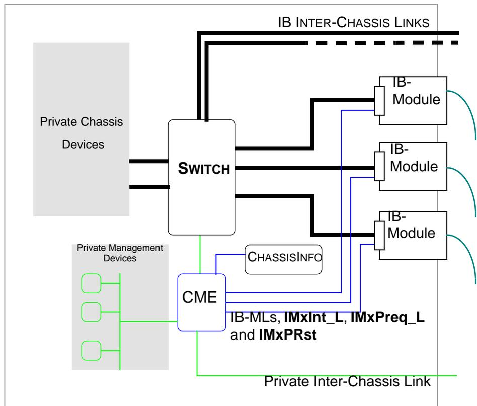
Figure 162 Actively Managed Chassis
