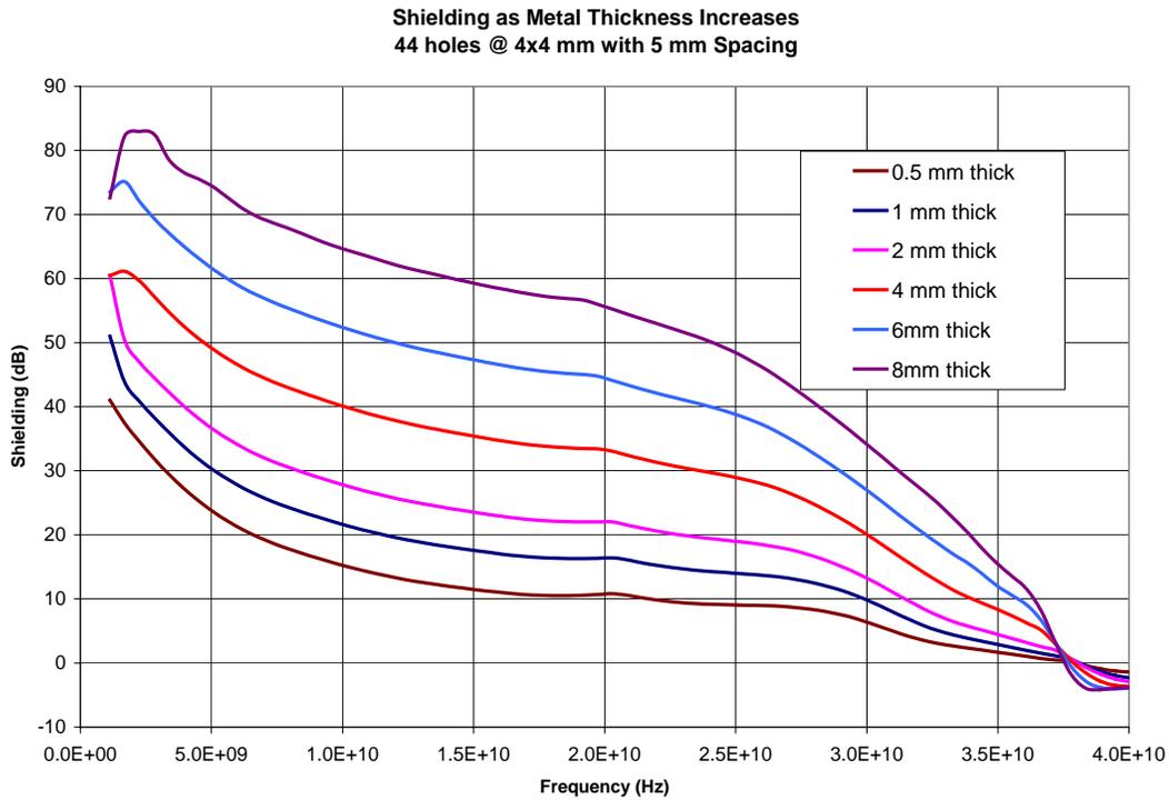
**Figure 195 44 Holes, 4x4 mm Square 5mm Center-to-Center**
