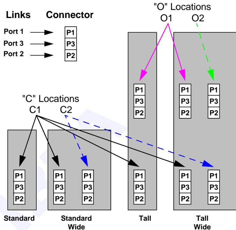
**Figure 6 Module Connector Location Designation**
