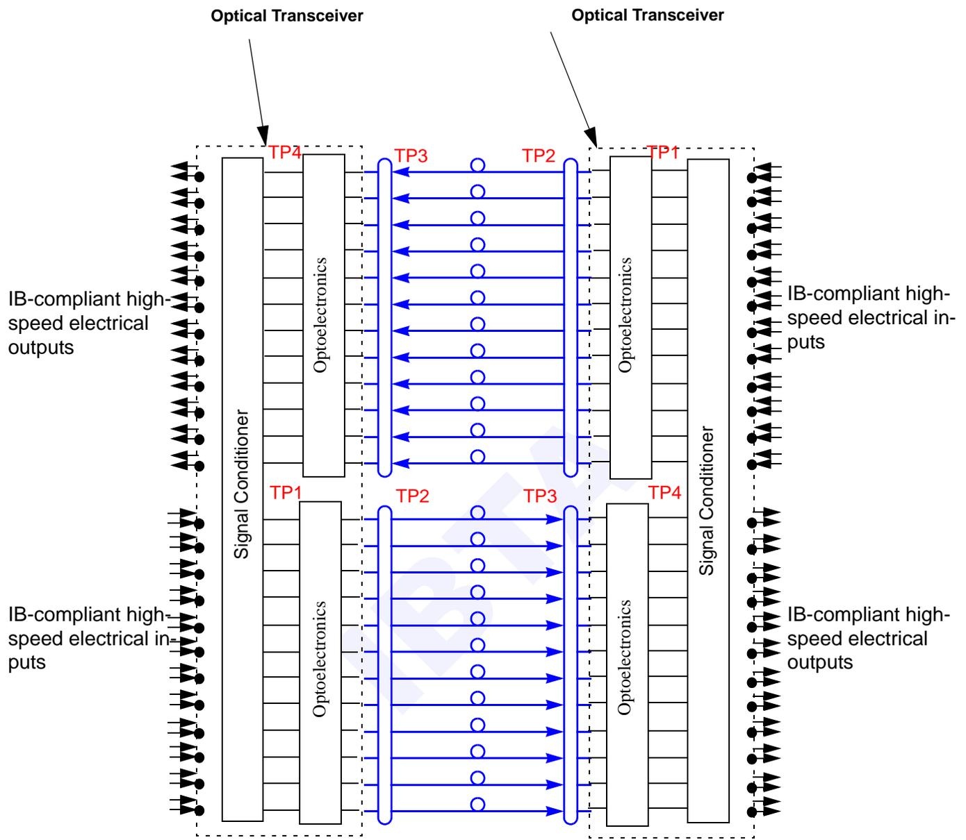
**Figure 91 Recommended 12x-SX & 12x-DDR-SX Optical Link Implementation**
