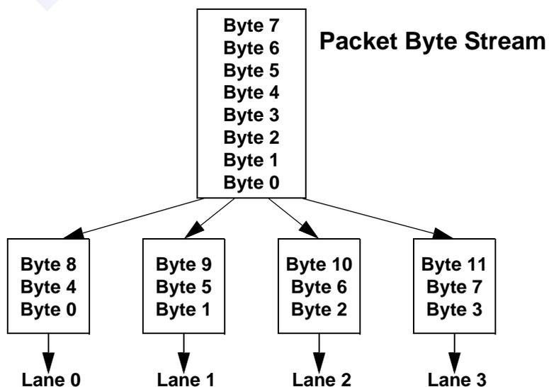
Figure 8 Example 4x Byte Striping Diagram
