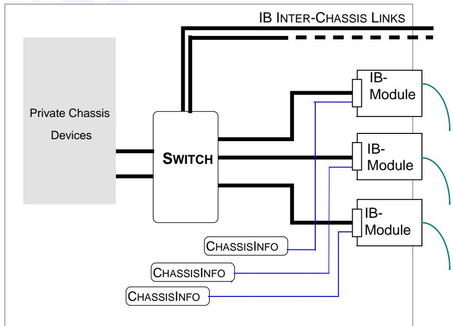
Figure 163 Passively Managed Chassis
