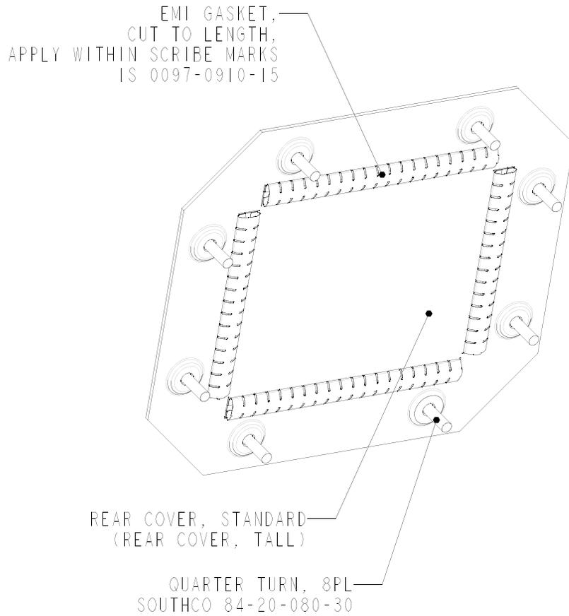
**Figure 210 Rear Cover Assembly - Standard; Tall**
