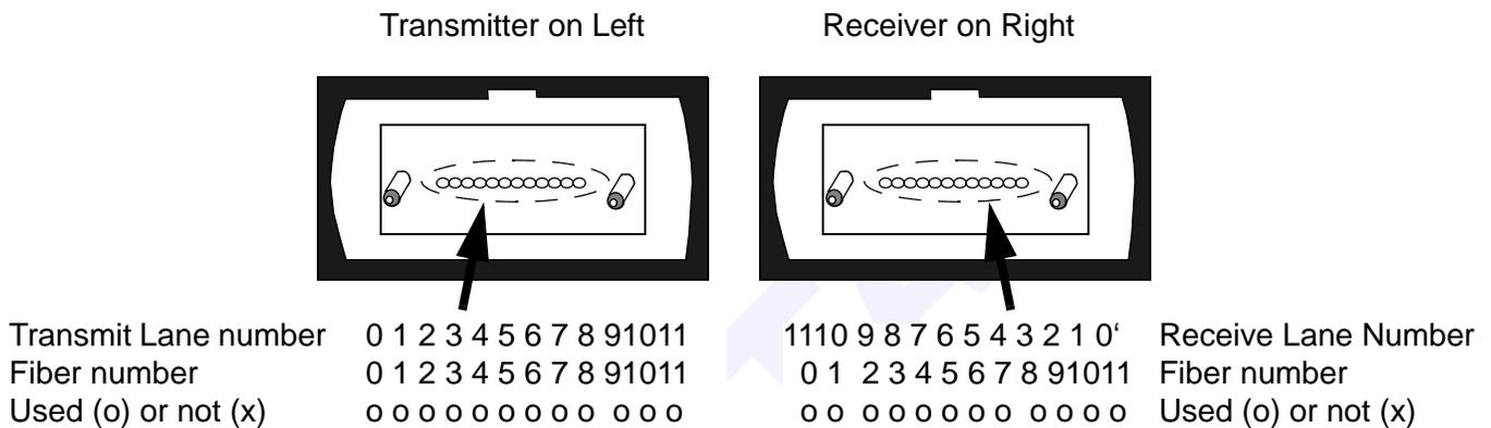
**Figure 86 12x-SX and 8x-SX Optical Receptacle orientation looking into the Transceiver**
