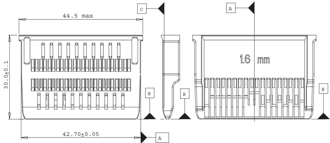
**Figure 132 Paddle guard, board primary, side and secondary views**
