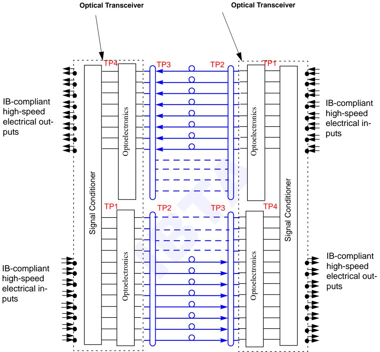
**Figure 90 Recommended 8x-SX and 8x-DDR-SX Optical Link Implementation**
