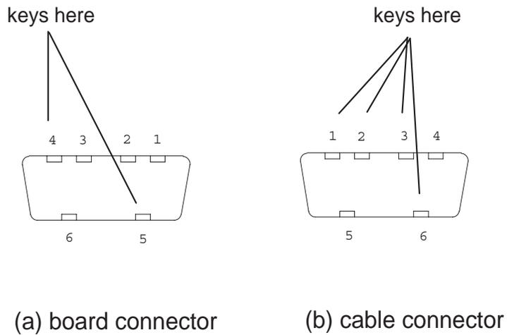
**Figure 50 4x board and cable connector keying**
