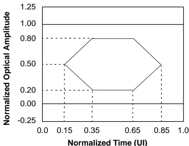
Figure 72 Normalized Optical Transmitter Compliance Mask
