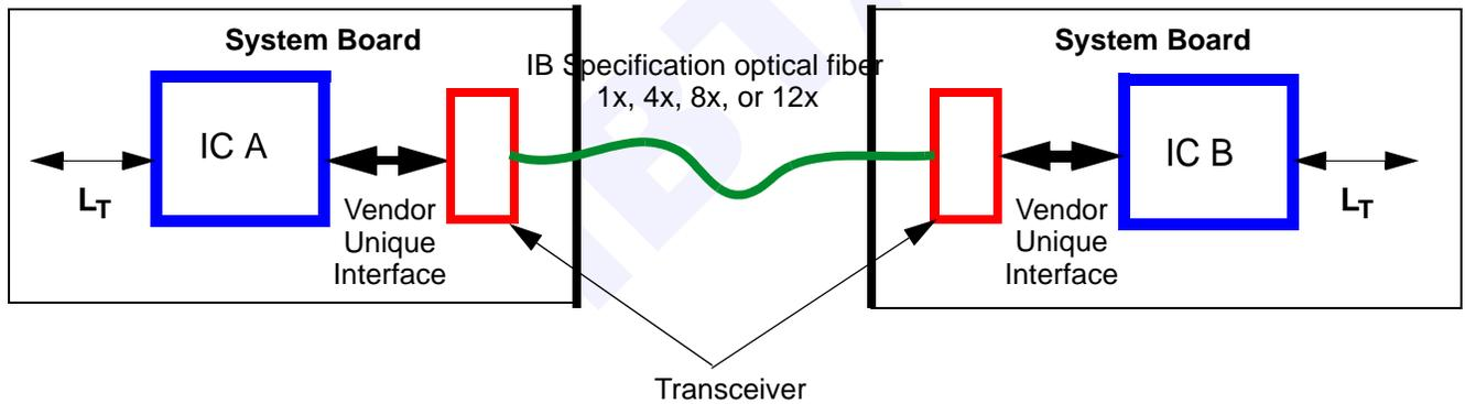
Figure 42 System Board Optical Fiber Interconnect Topology
