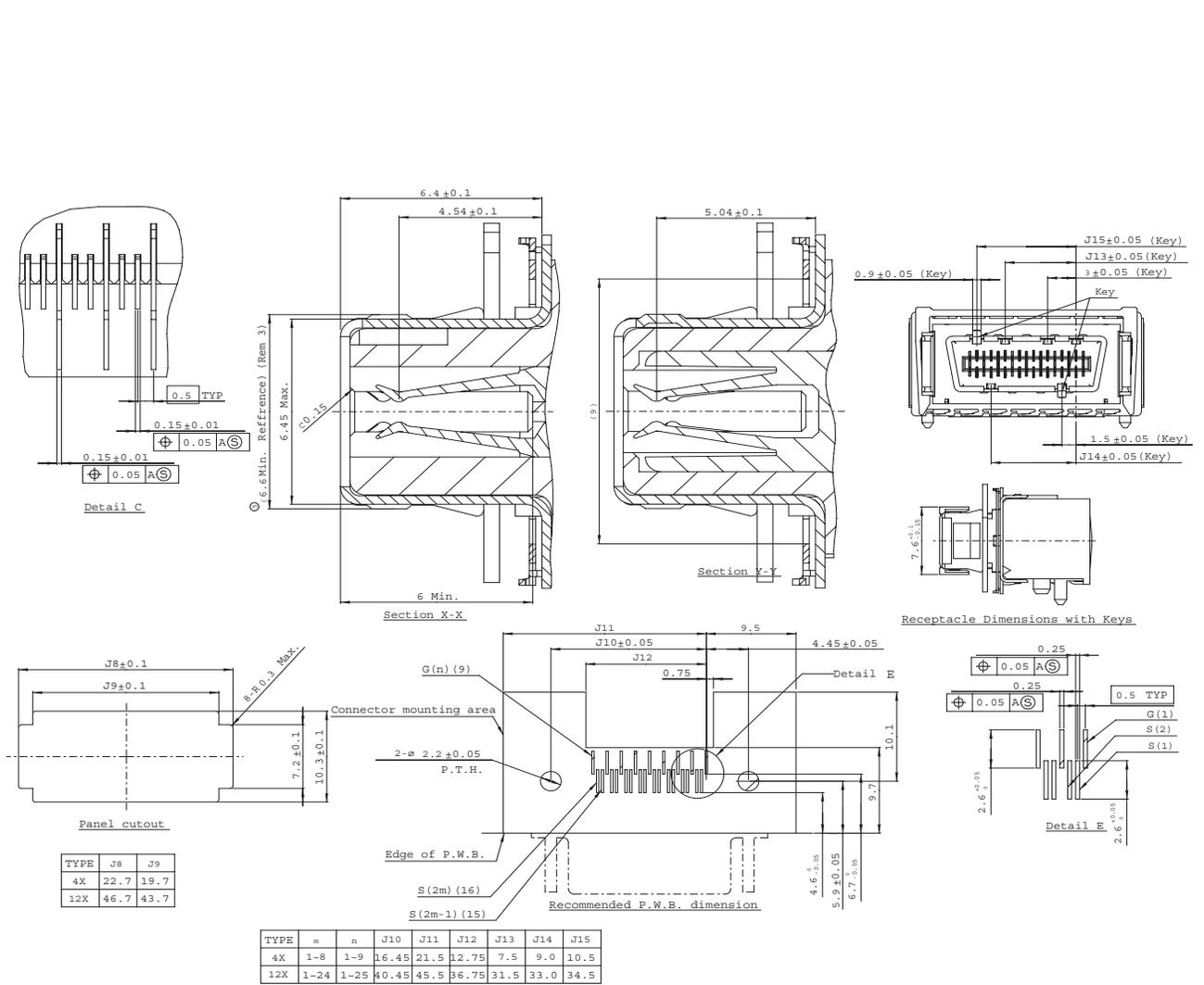
Figure 48 4x/12x cable board connector interface details
