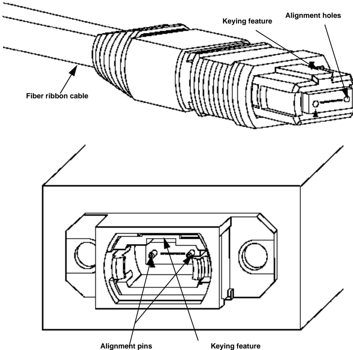
**Figure 81 MPO Plug and Receptacle**
