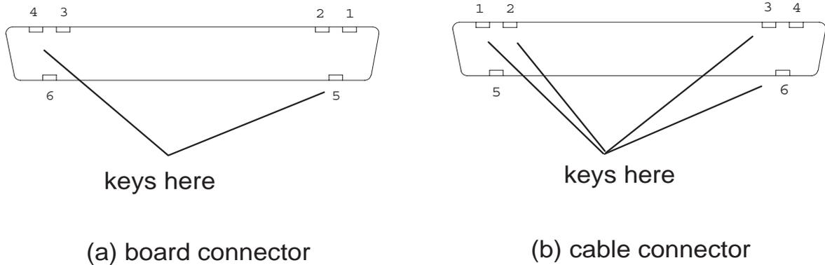
**Figure 53 12x board and cable connector keying**
