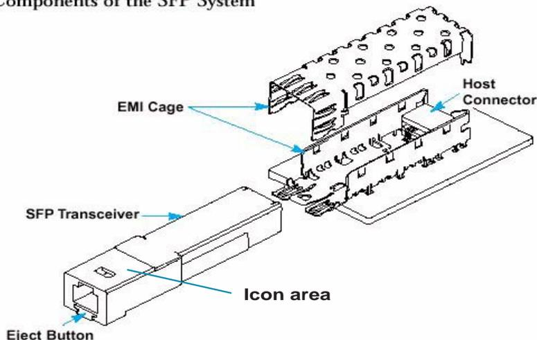
Figure 54 1x Pluggable interface and transceiver assembly
