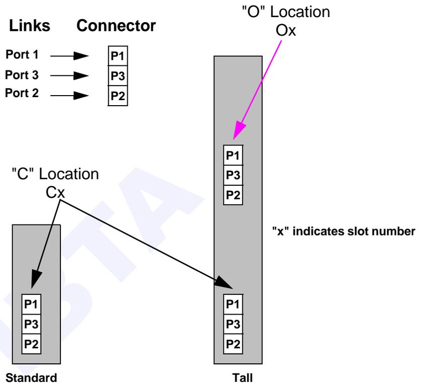
Figure 7 Chassis Connector Location Designation
