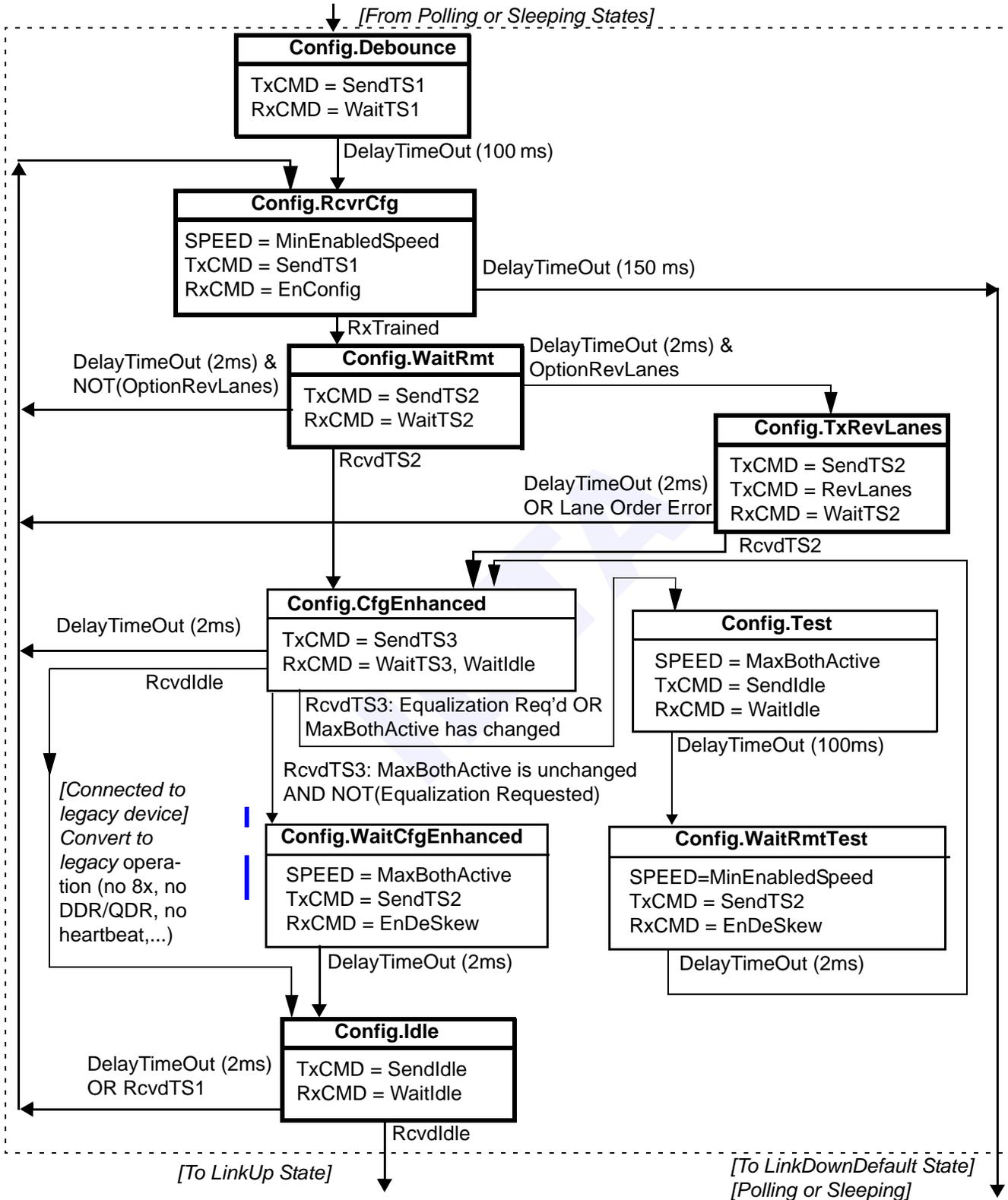
Figure 26 Configuration Super State (Expanded) - Enhanced Signaling
