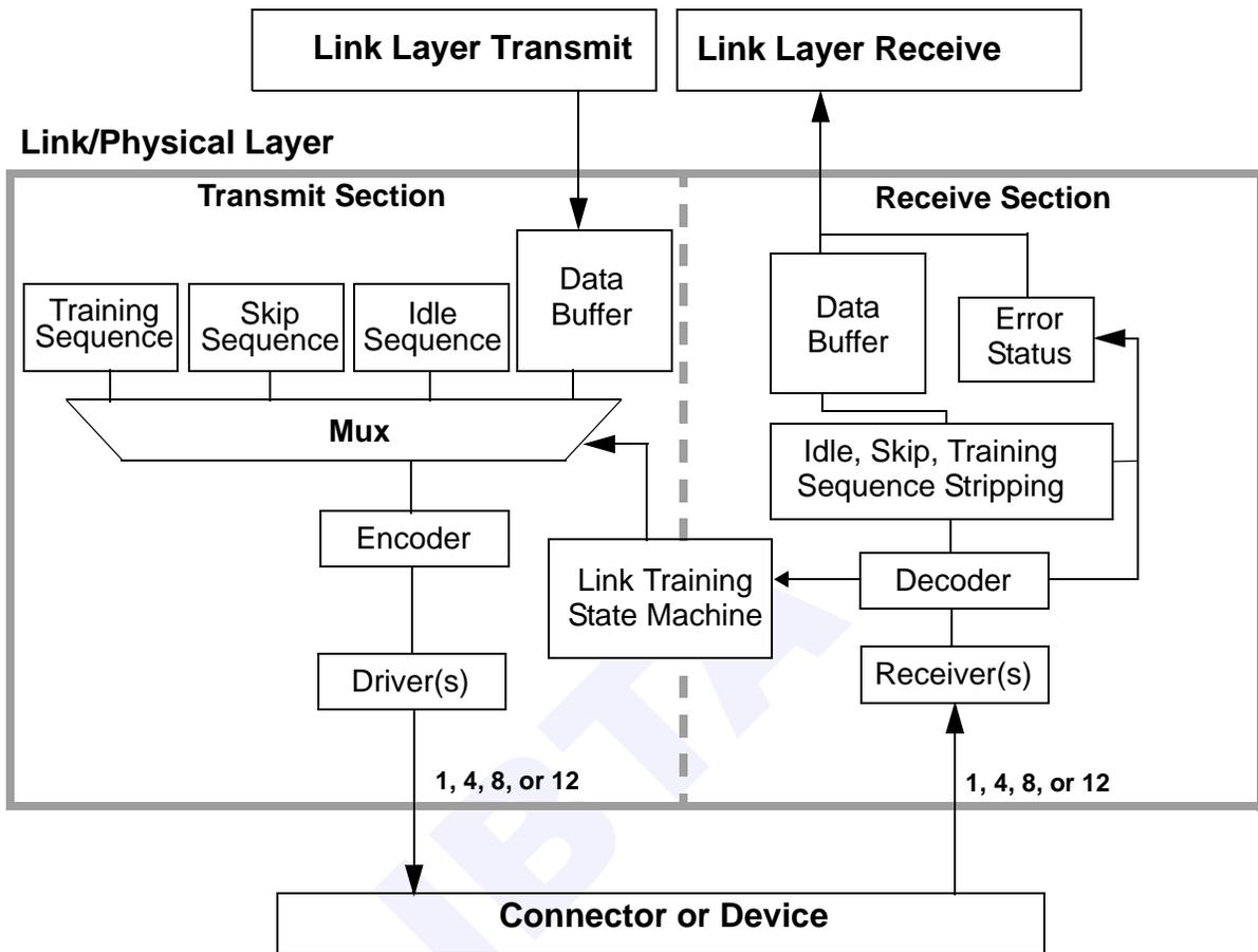
Figure 9 Link/Physical Interface Block Diagram
