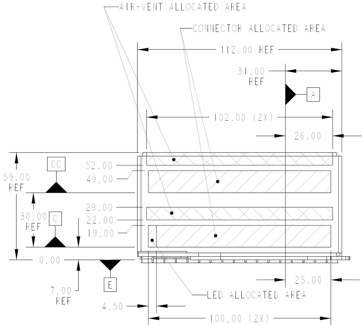
**Figure 107 Wide Critical Dimensions - Detail C**
