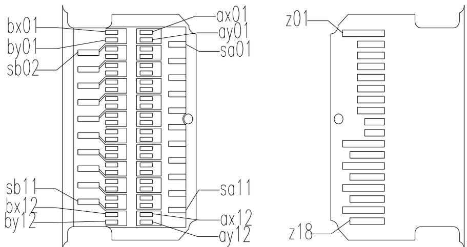
**Figure 136 Board contact assignment, primary and secondary sides**
