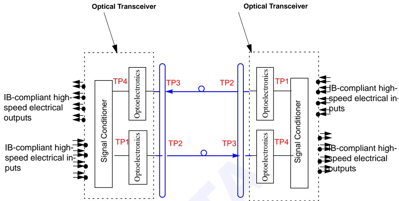
**Figure 89 Recommended 4x-LX Optical Link Implementation**
