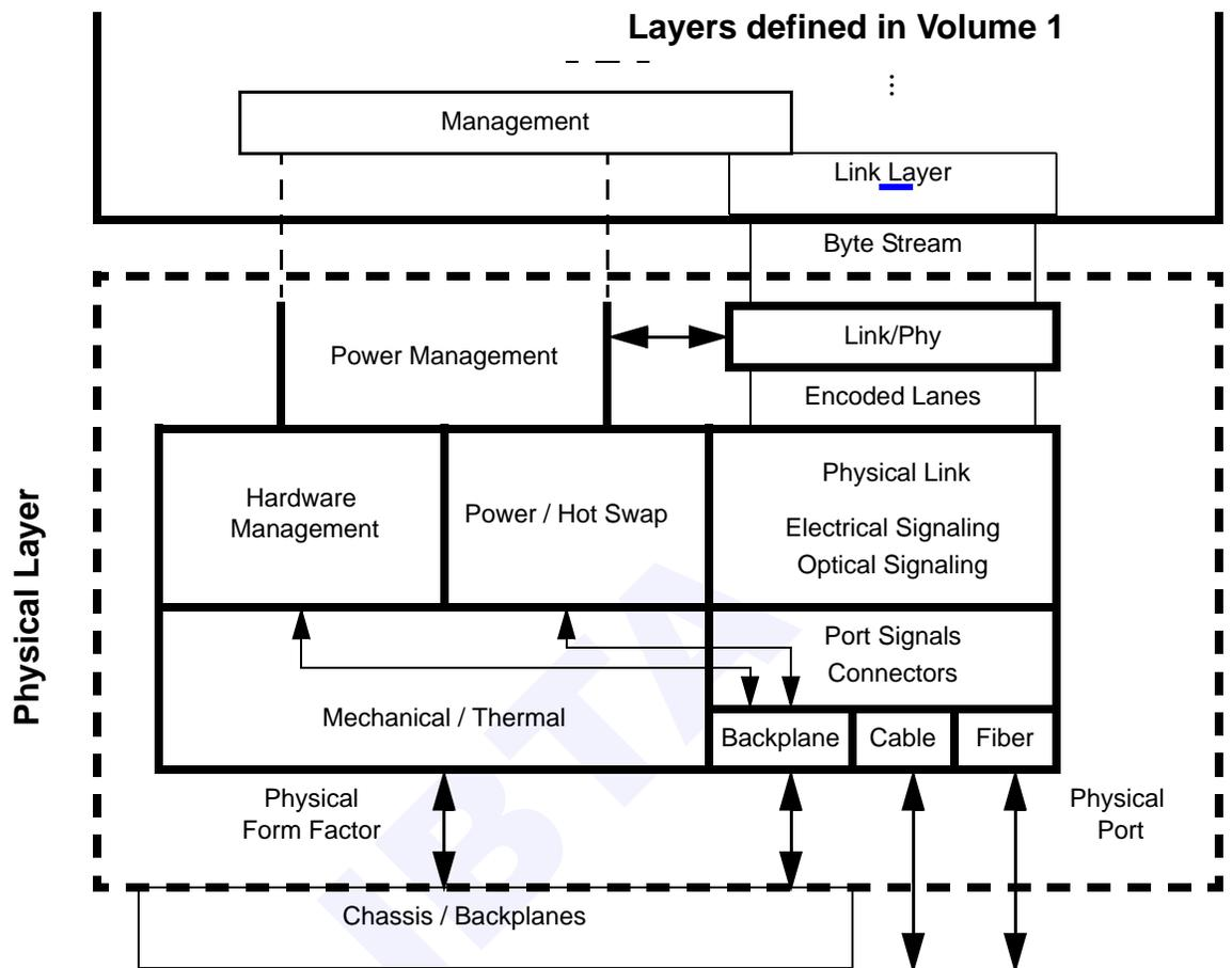
**Figure 1 Physical Layer Structure**
