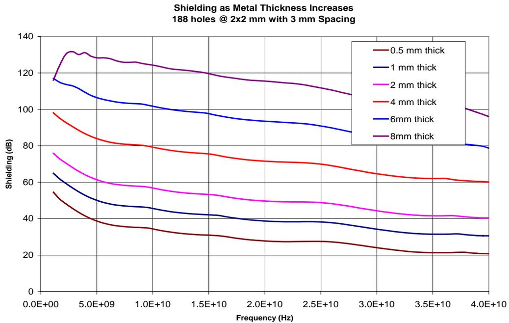
**Figure 194 188 Holes, 2x2 mm Square 3mm Center-to-Center**
