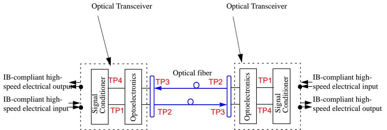
**Figure 87 Recommended 1x, 1x DDR, and 1x QDR Optical Link Implementation**
