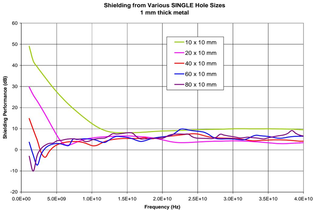
**Figure 198 Shielding Performance: Single Hole, Various Sizes, 1mm Thick**
