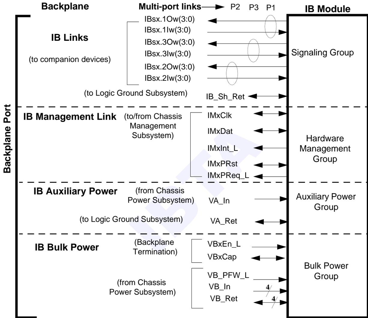
Figure 5 Backplane Port - Multiple Physical Links
