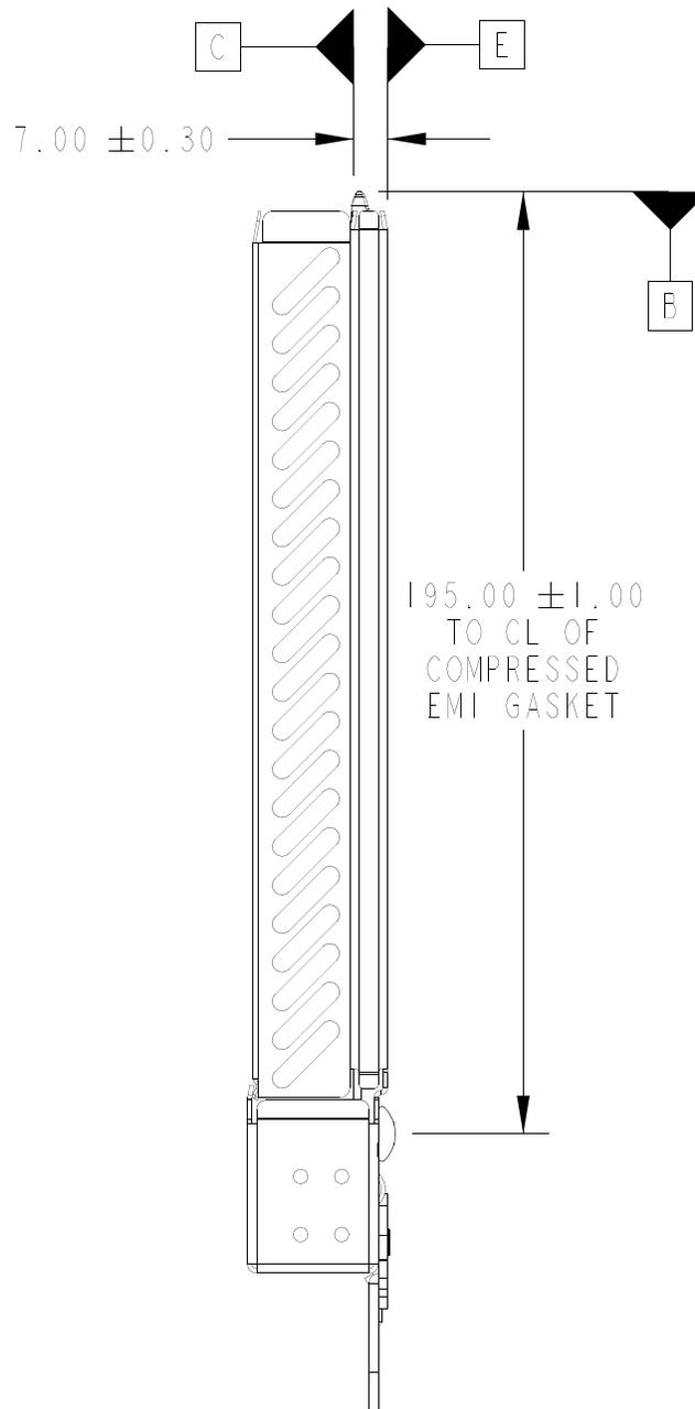
Figure 98 Standard Critical Dimensions - Detail B
