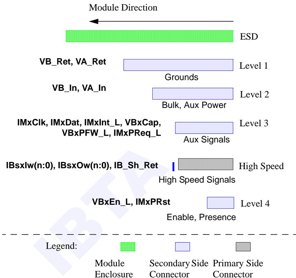
**Figure 155 Module Insertion Contact Sequence**
