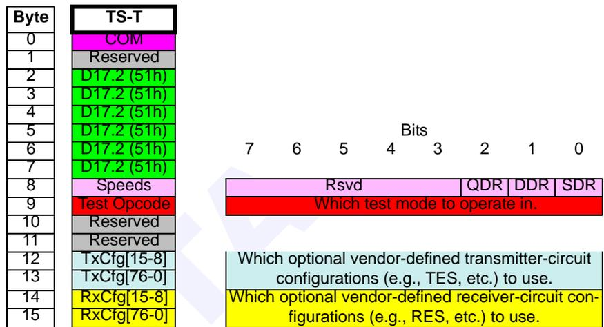
**Figure 14 TS-T Ordered-Set: Detailed Format**
