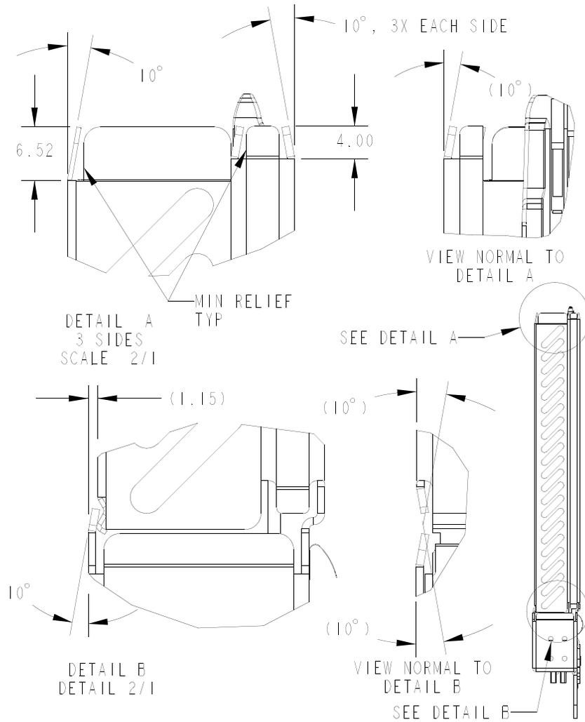
**Figure 112 Module Lead-in Features, Standard Module**
