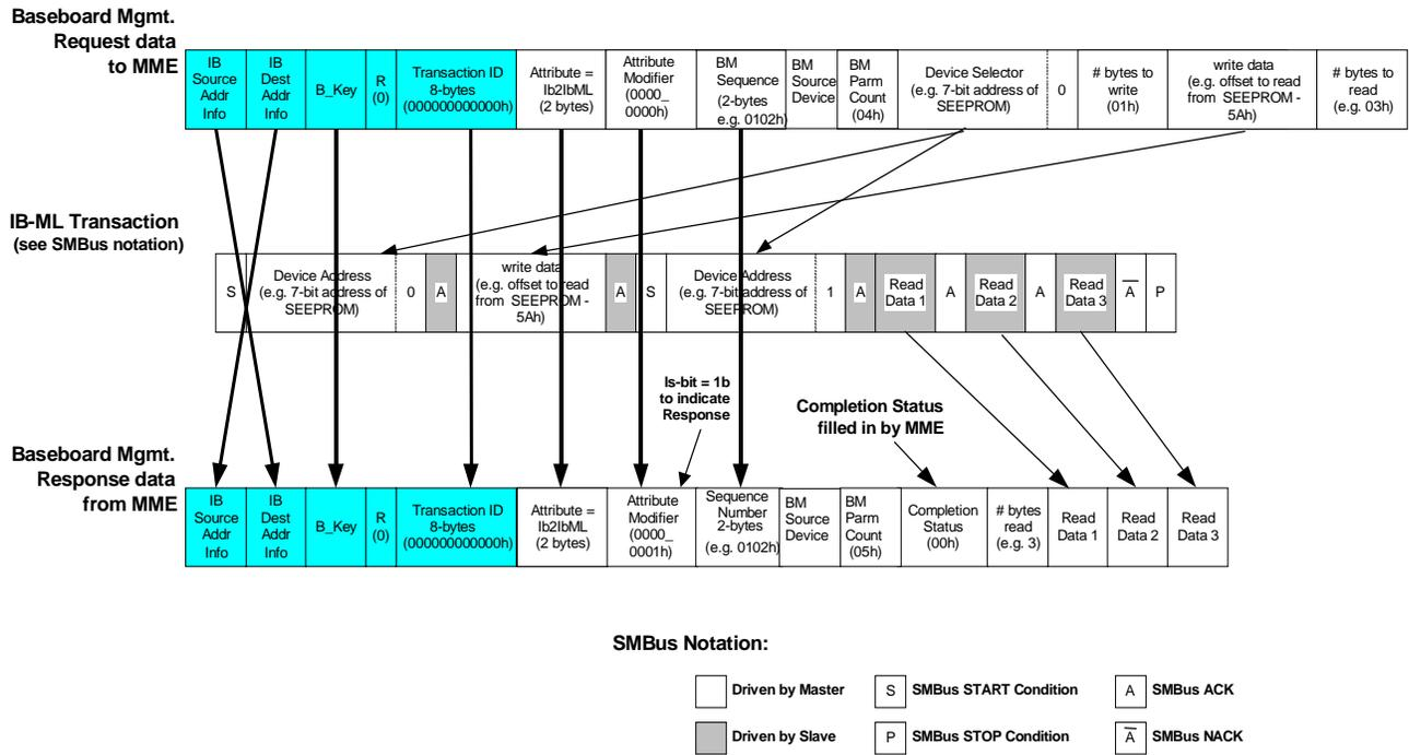
Figure 168 IB-to-IB-ML Access
