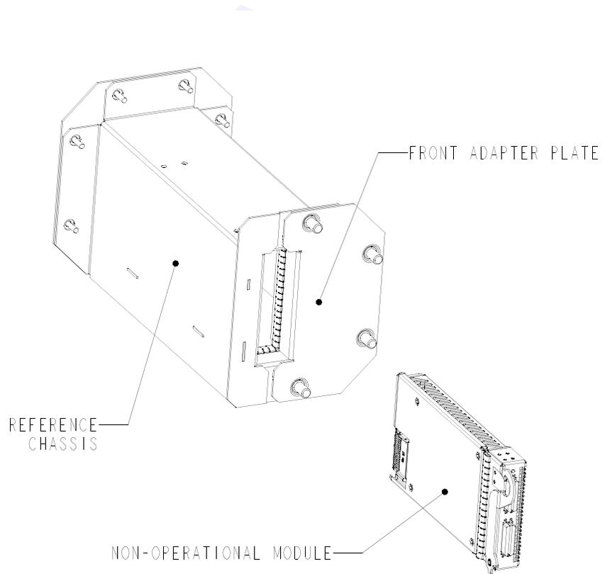
**Figure 203 Attenuation Reference Chassis and Standard Module**
