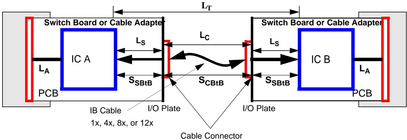
**Figure 39 I/O Plate to I/O Plate via Cable Topology**
