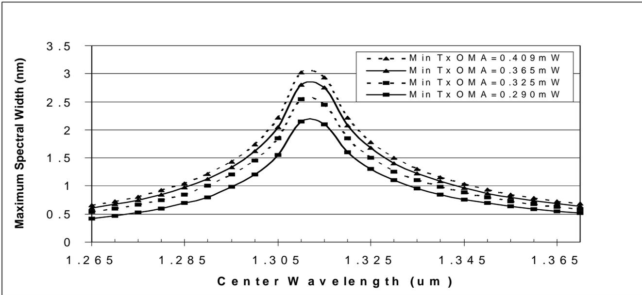
Figure 77 1x-DDR-LX Trade-off between OMA, RMS Spectral Width, and Center Wavelength
