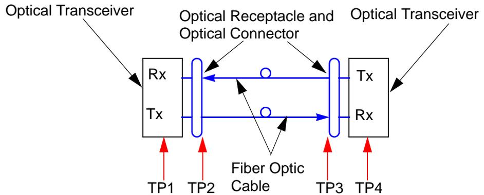
For clarity, only the jitter compliance test points for the left-to-right portion of the link are shown
