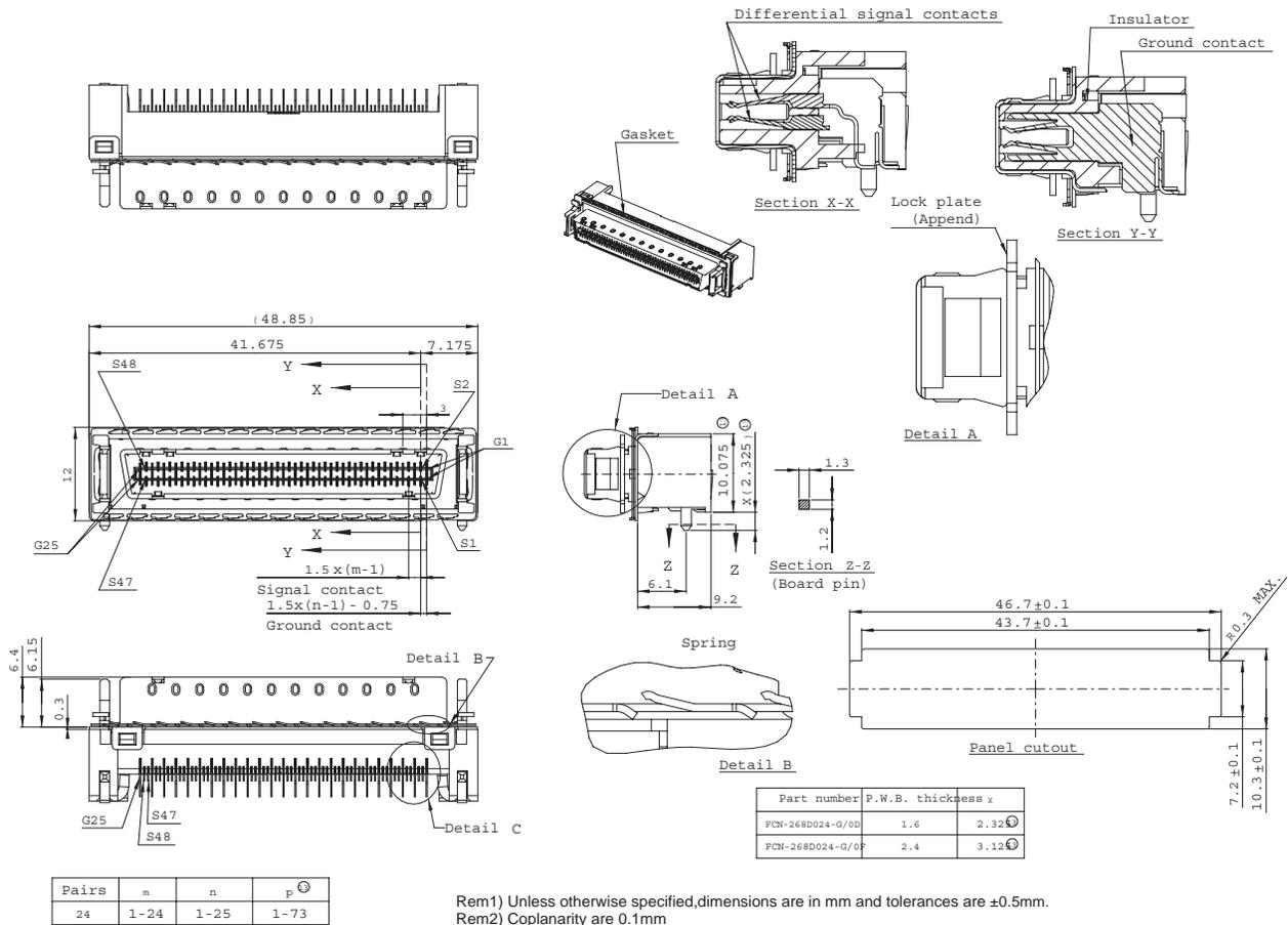
Figure 51 12x cable board connector
