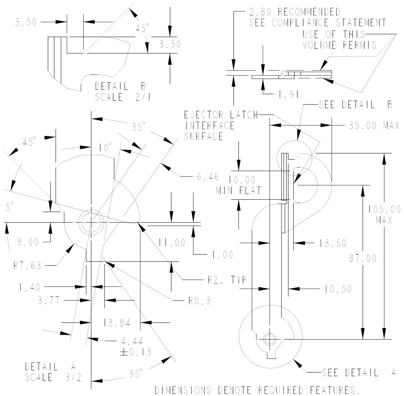
Figure 115 Standard Ejector Dimensions
