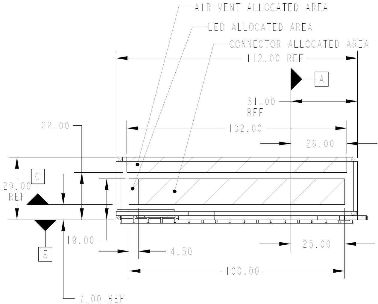
Figure 99 Standard Critical Dimensions - Detail C
