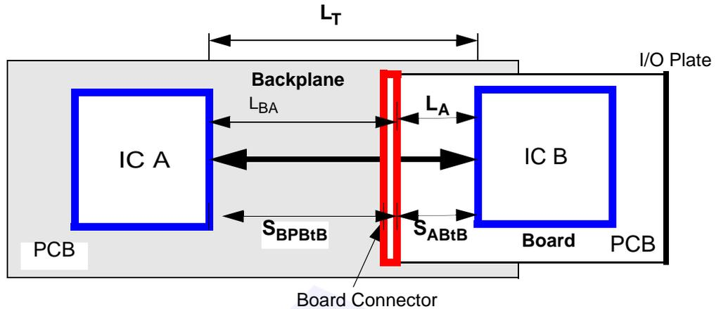
Figure 37 Slot on Active Backplane Topology
