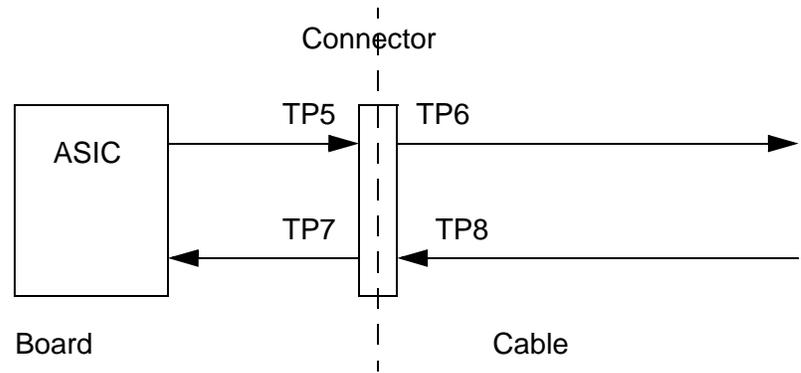
Figure 34 Board/Cable test points
