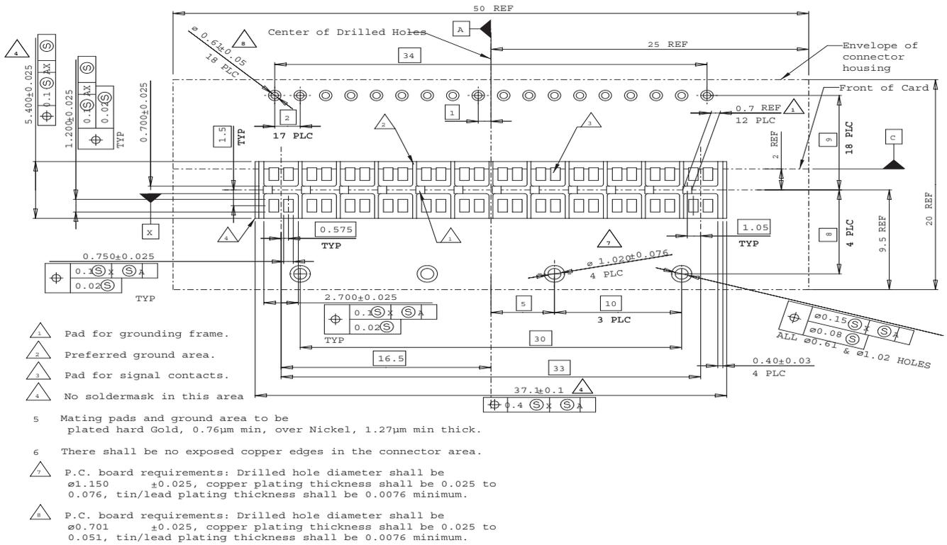
**Figure 139 Backplane connector footprint for 12x port**
