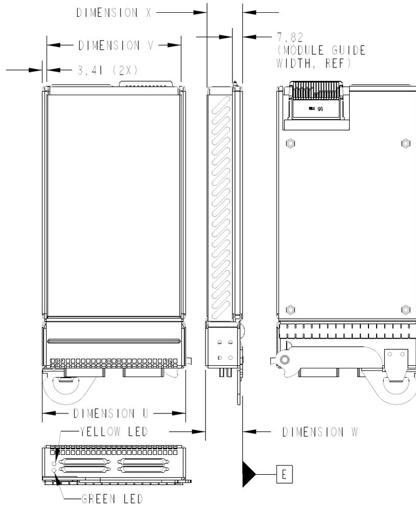
**Figure 95 General Module Assembly Dimensions (Parametric)**
