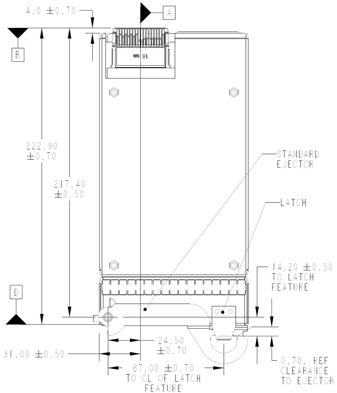
Figure 97 Standard Critical Dimensions - Detail A
