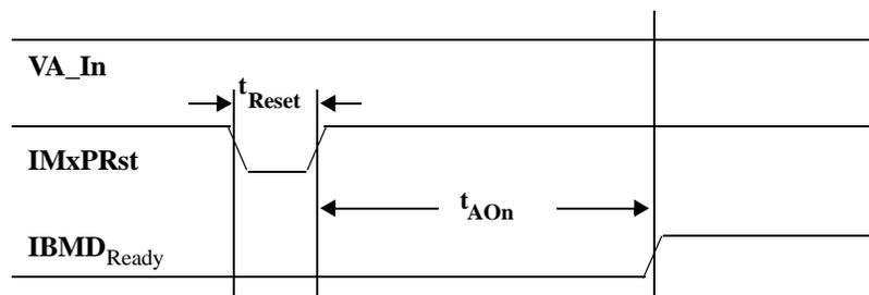
Figure 151 IMxPRst Timing Measurements
