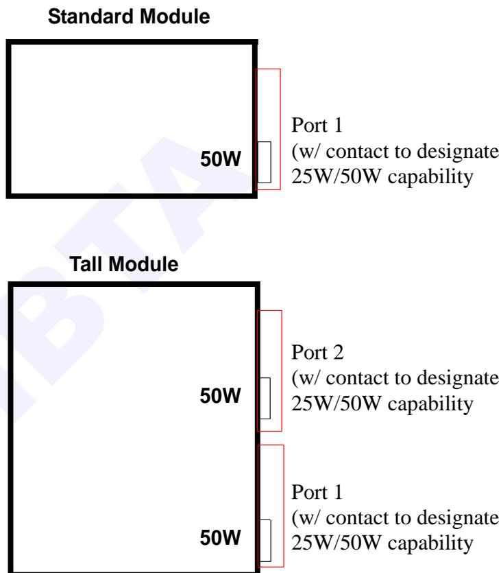
Figure 154 Module Bulk Power Ports (Logical)
