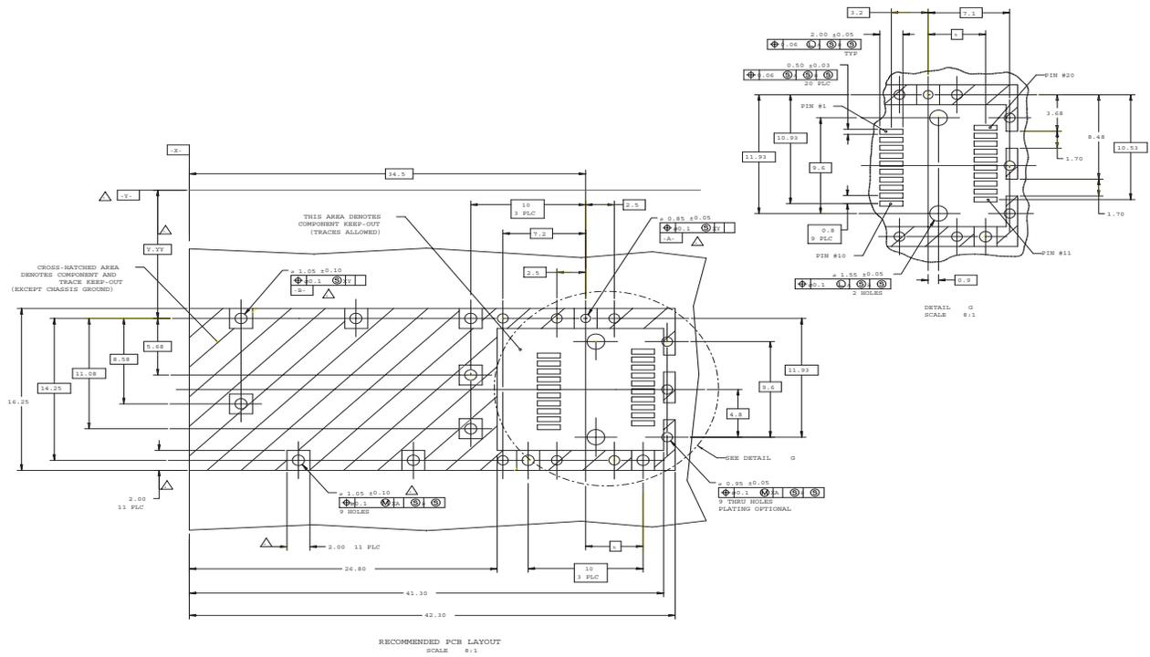
Figure 55 Pluggable interface board connector footprint
