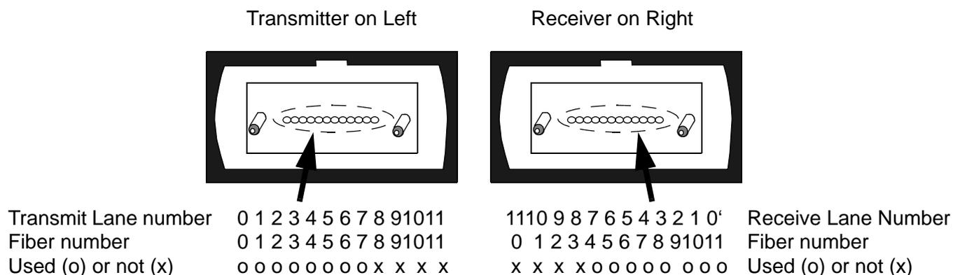
**Figure 84 8x-SX Optical Receptacle orientation looking into the Transceiver**
