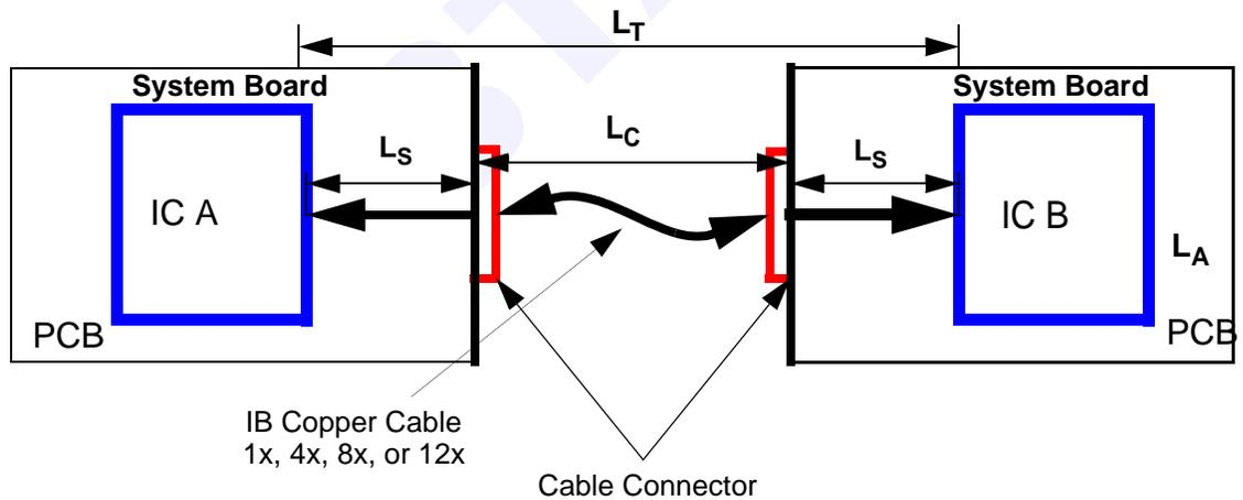
**Figure 40 System Board to System Board via Cable Topology**
