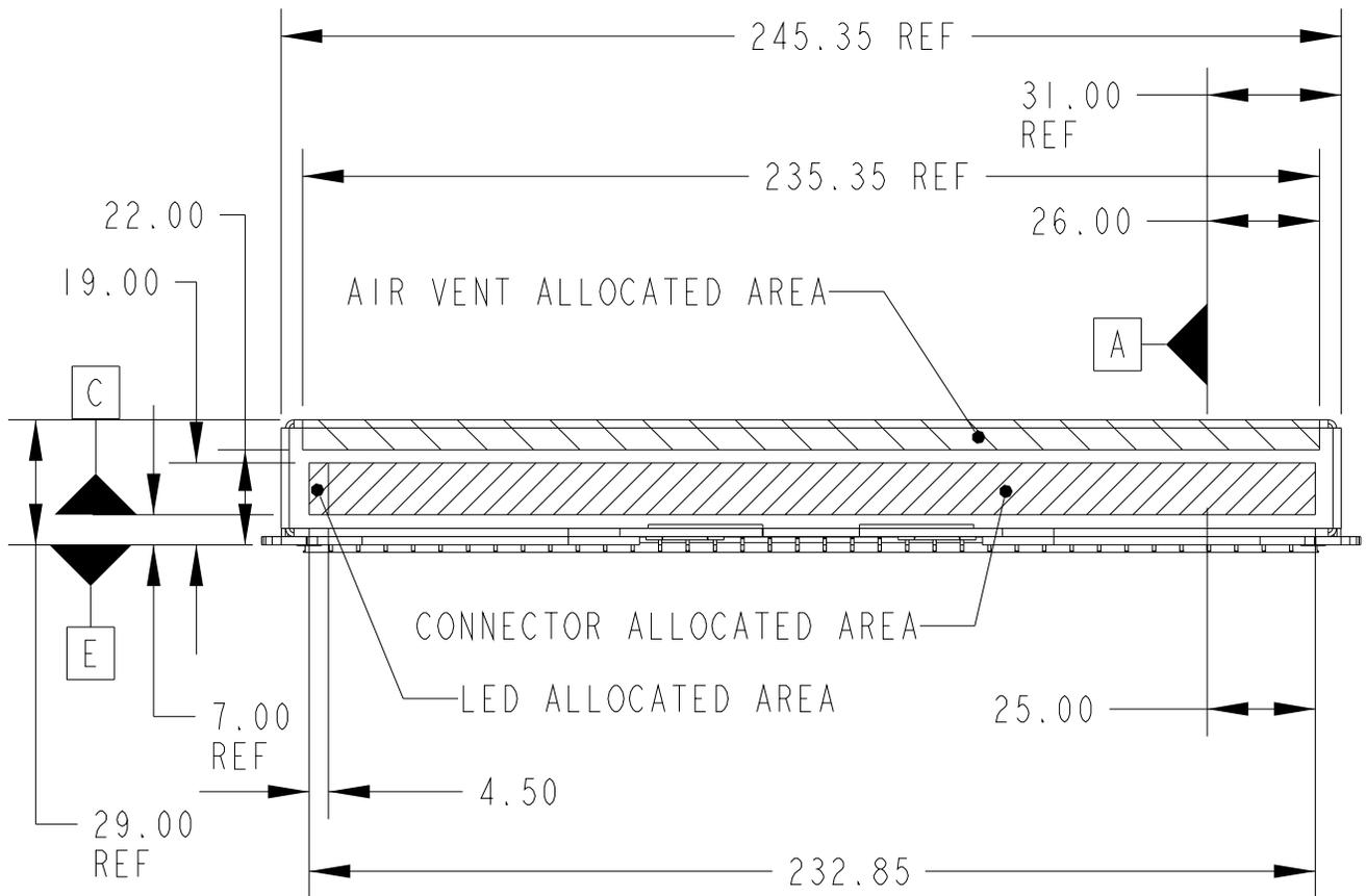
Figure 103 Tall Critical Dimensions - Detail C
