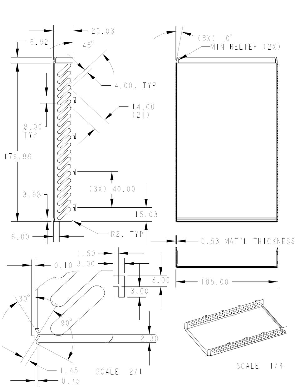
Figure 183 IB Cover Example
