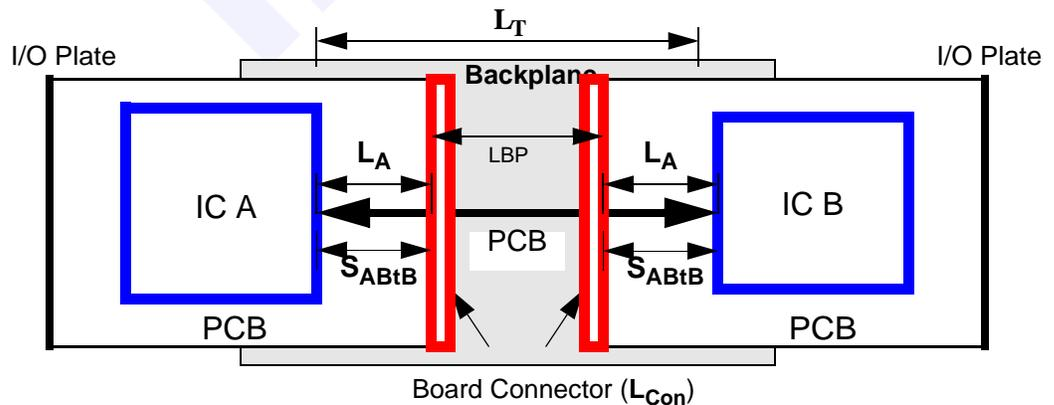
Figure 38 Slot to Slot on Passive Backplane Topology
