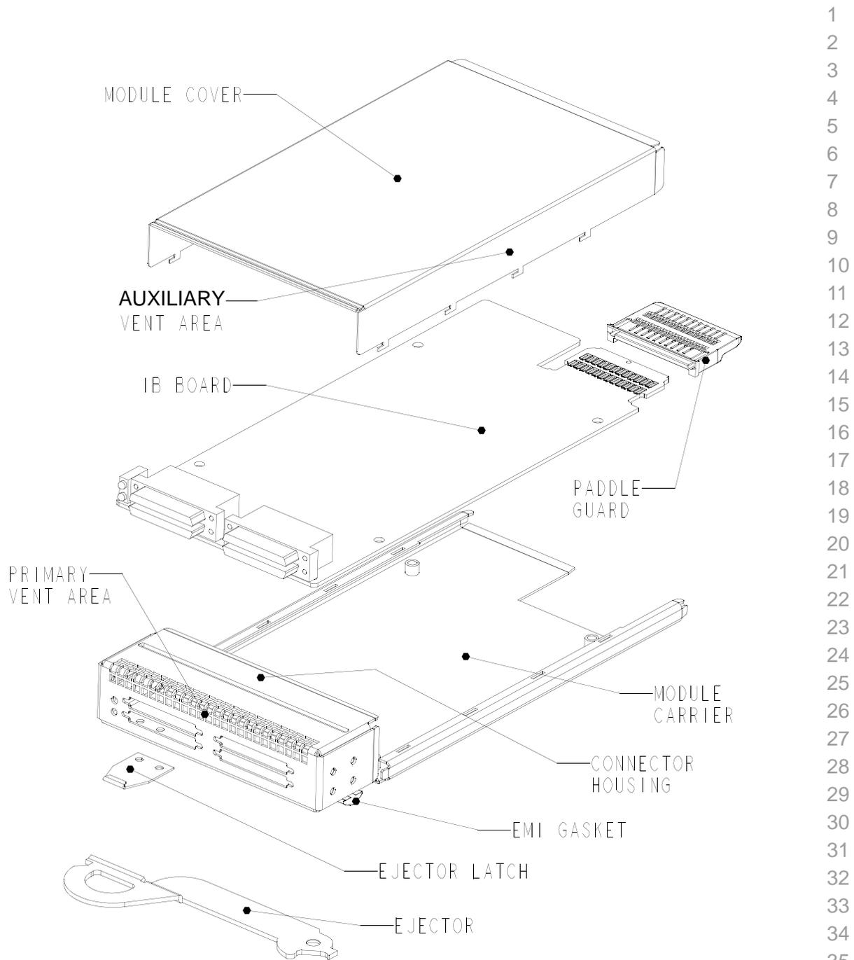
**Figure 93 Exploded View of InfiniBand Standard Module**
