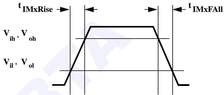
Figure 150 IMxPRst, IMxInt, IMxPREq\_L Timing Measurements
