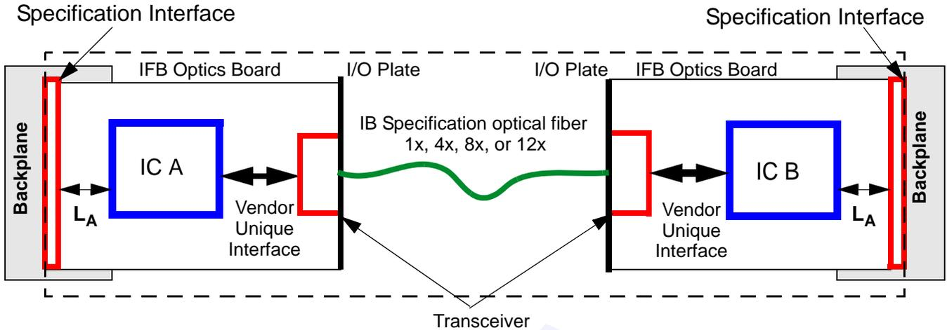
Figure 41 Optical Fiber Interconnect Topology
