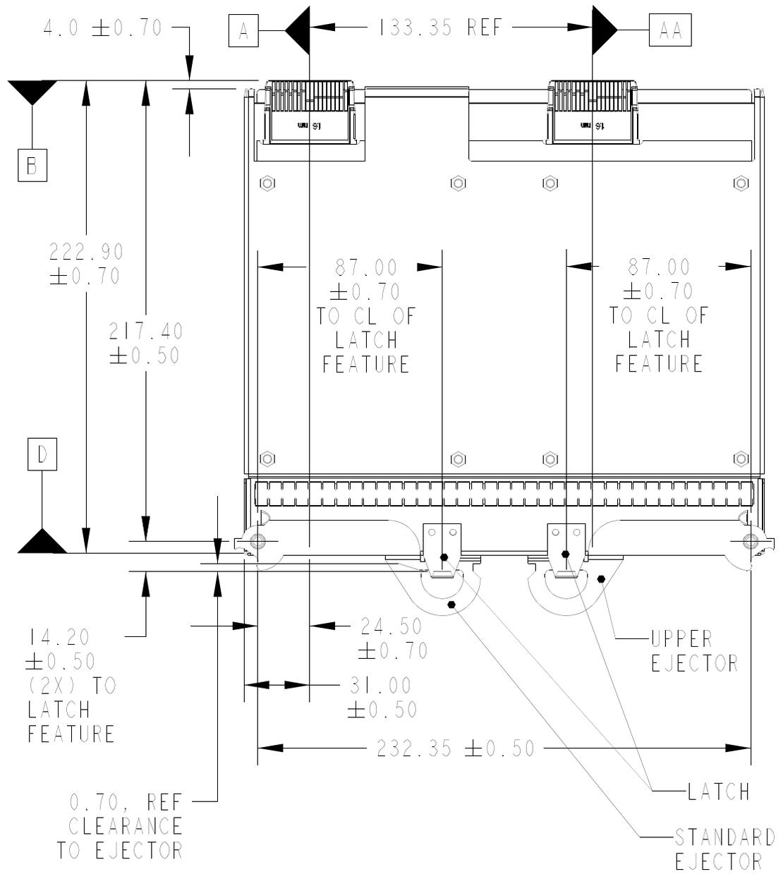
Figure 101 Tall Critical Dimensions - Detail A
