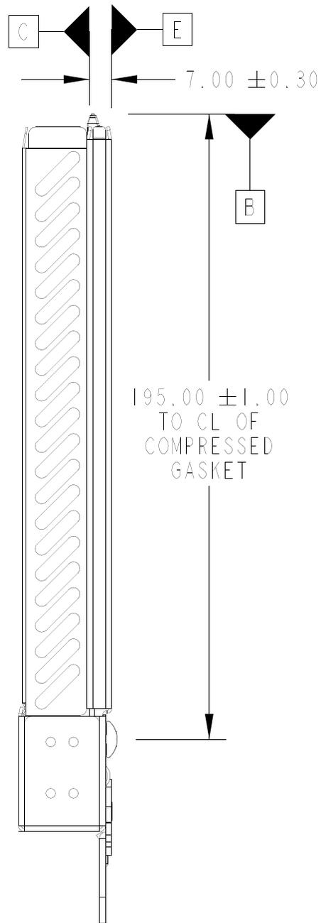
Figure 102 Tall Critical Dimensions - Detail B
