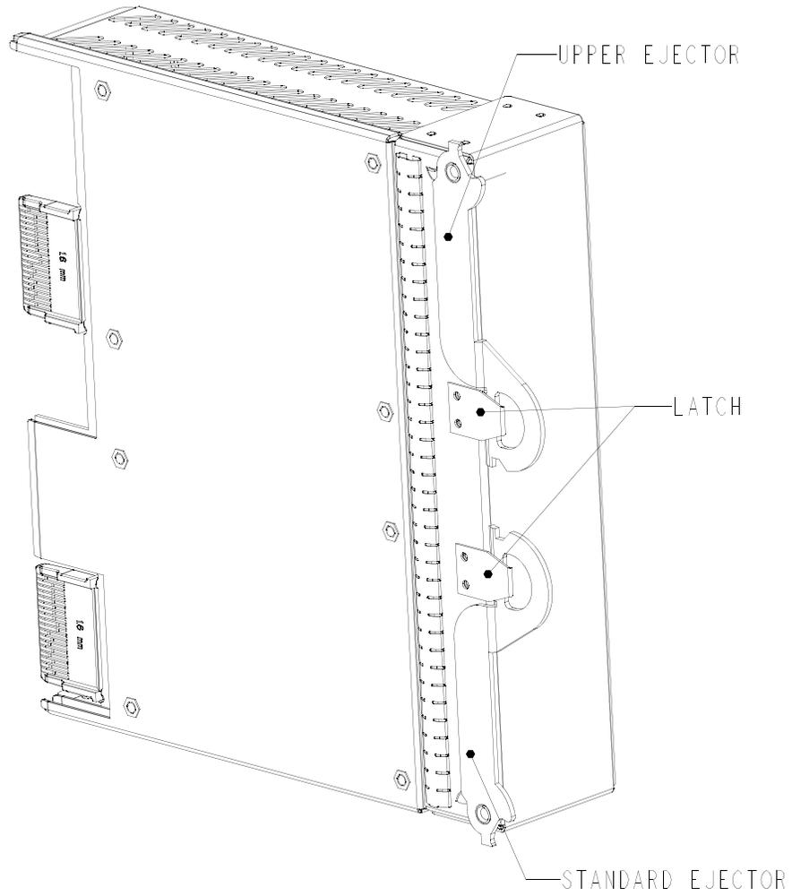
**Figure 114 Tall Wide Module With Ejectors and Latches**
