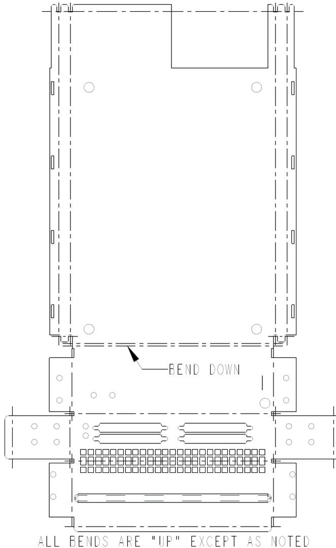
**Figure 189 Example IB Carrier Flat Pattern**
