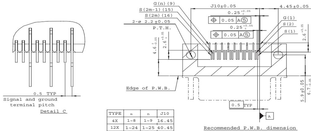
**Figure 49 4x cable board connector footprint, top view**
