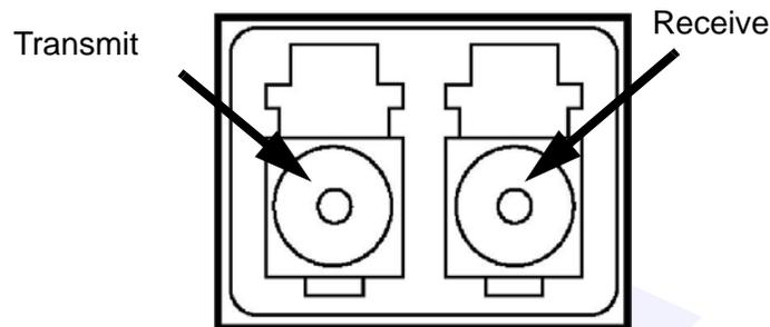
**Figure 80 1x-SX and 1x-LX Optical Receptacle orientation looking into the Optical Transceiver**
