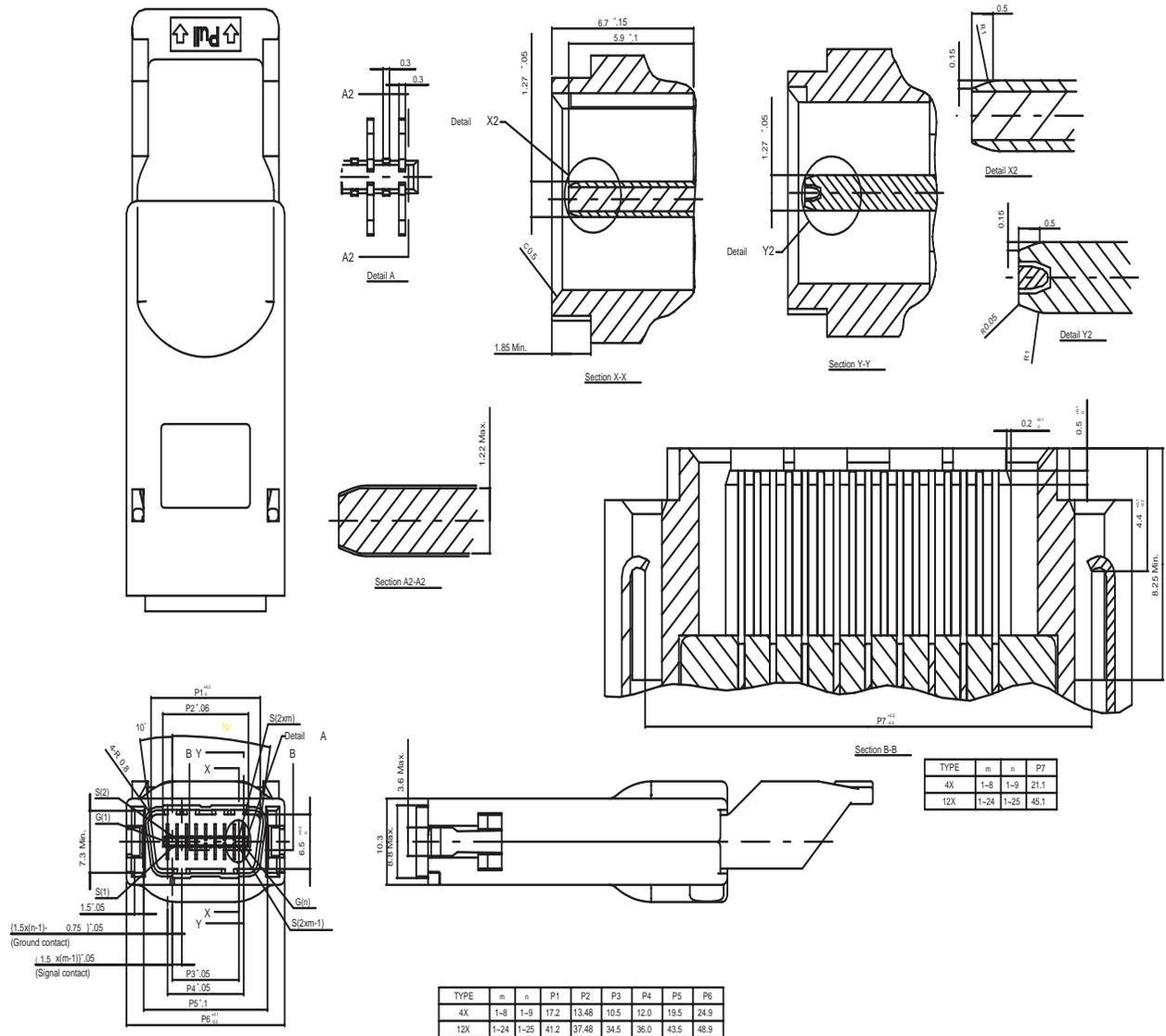
Figure 63 4x/12x cable plug interface details
