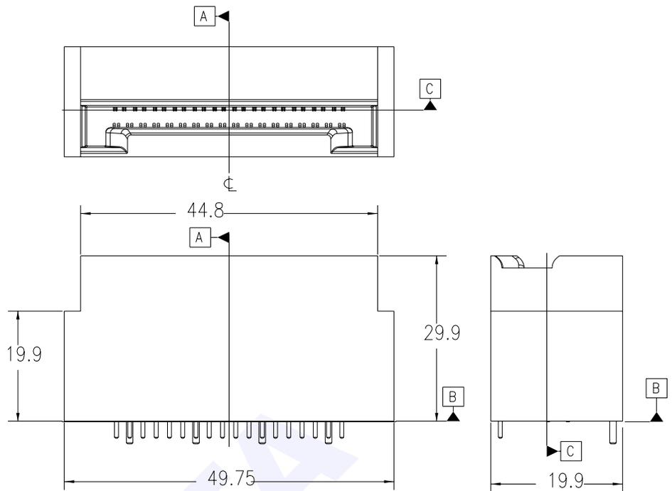
**Figure 137 Compression/press-fit backplane connector housing**
