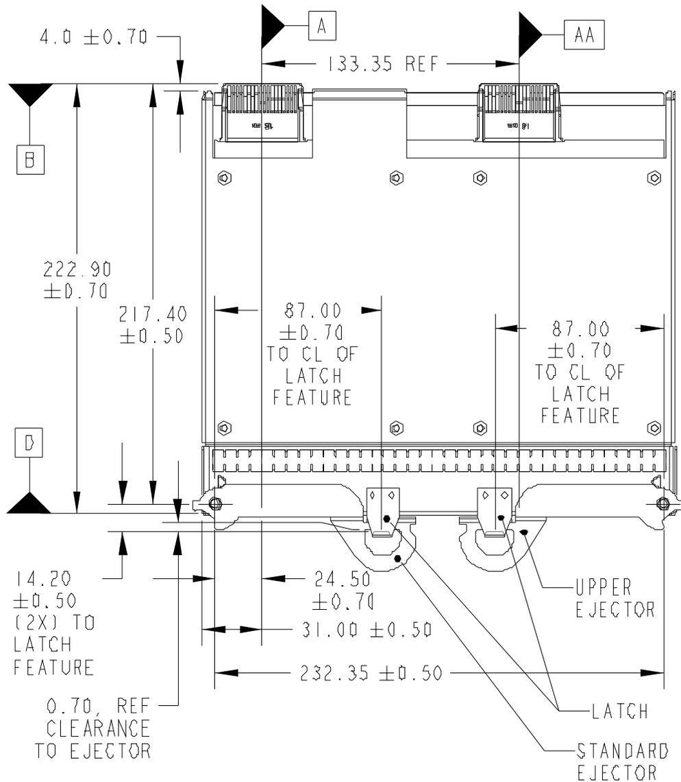
Figure 109 Tall Wide Critical Dimensions - Detail A
