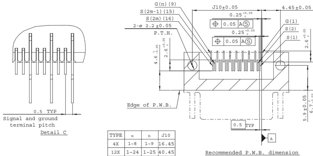
Figure 52 12x cable board connector footprint, top view
