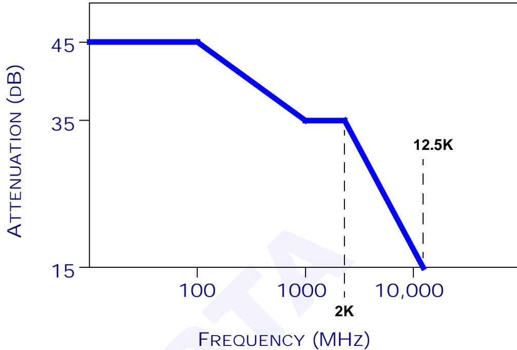
Figure 124 Required Carrier Attenuation
