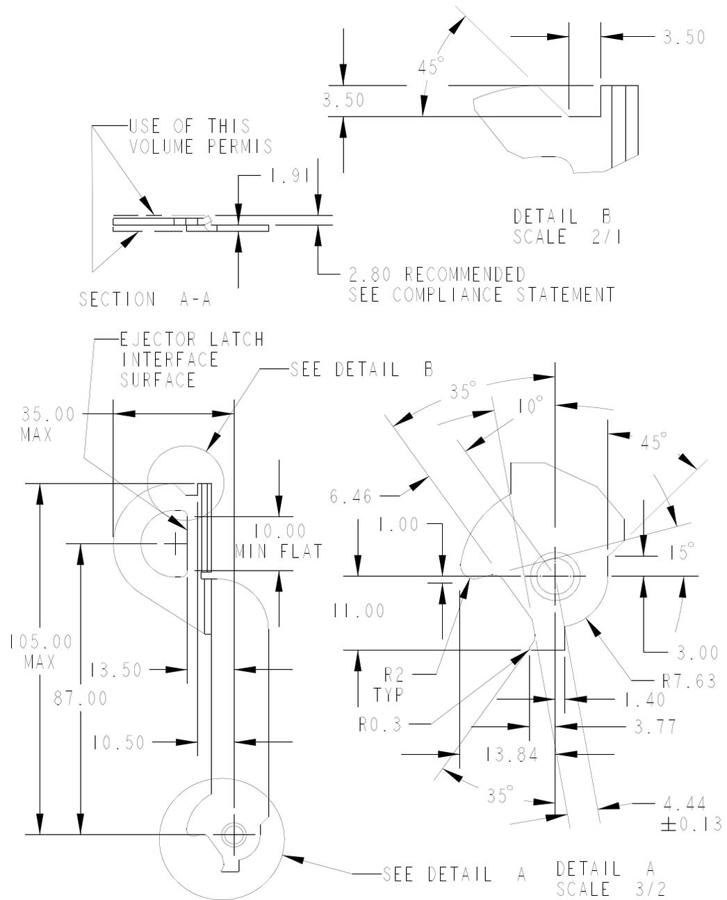
Figure 116 Upper Ejector Dimensions
