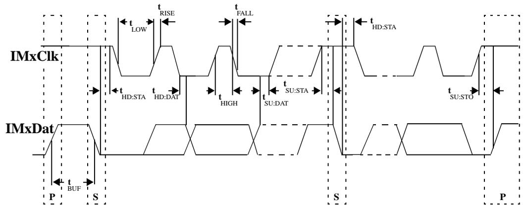
Figure 149 IMxDat, IMxClk Timing Measurements
