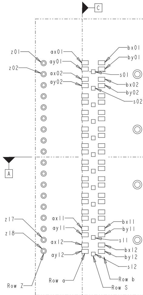
Figure 140 Backplane signal contact assignment, 12x port
