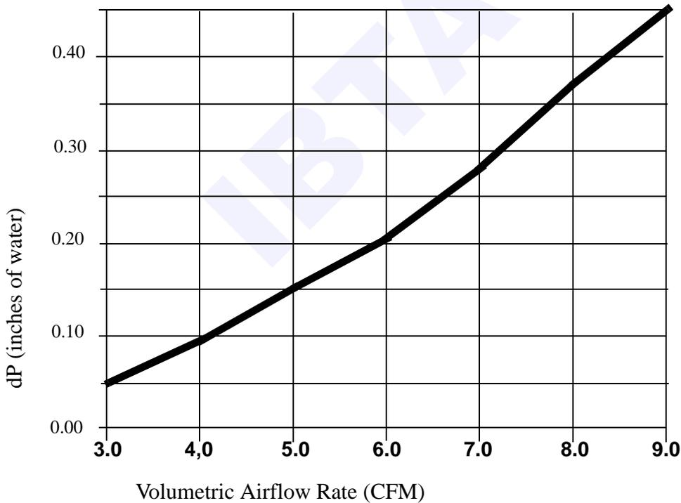
**Figure 193 Nozzle calibration curve for standard module**
