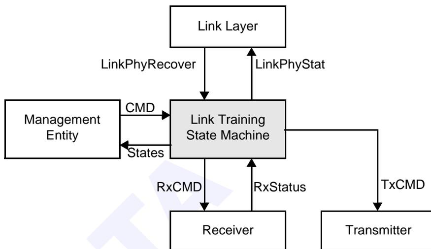
**Figure 20 Link Training State Machine Interactions**
