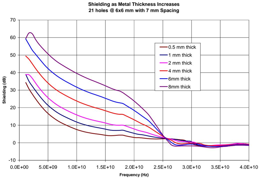
**Figure 196 21 Holes, 6x6 mm Square 7mm Center-to-Center**
