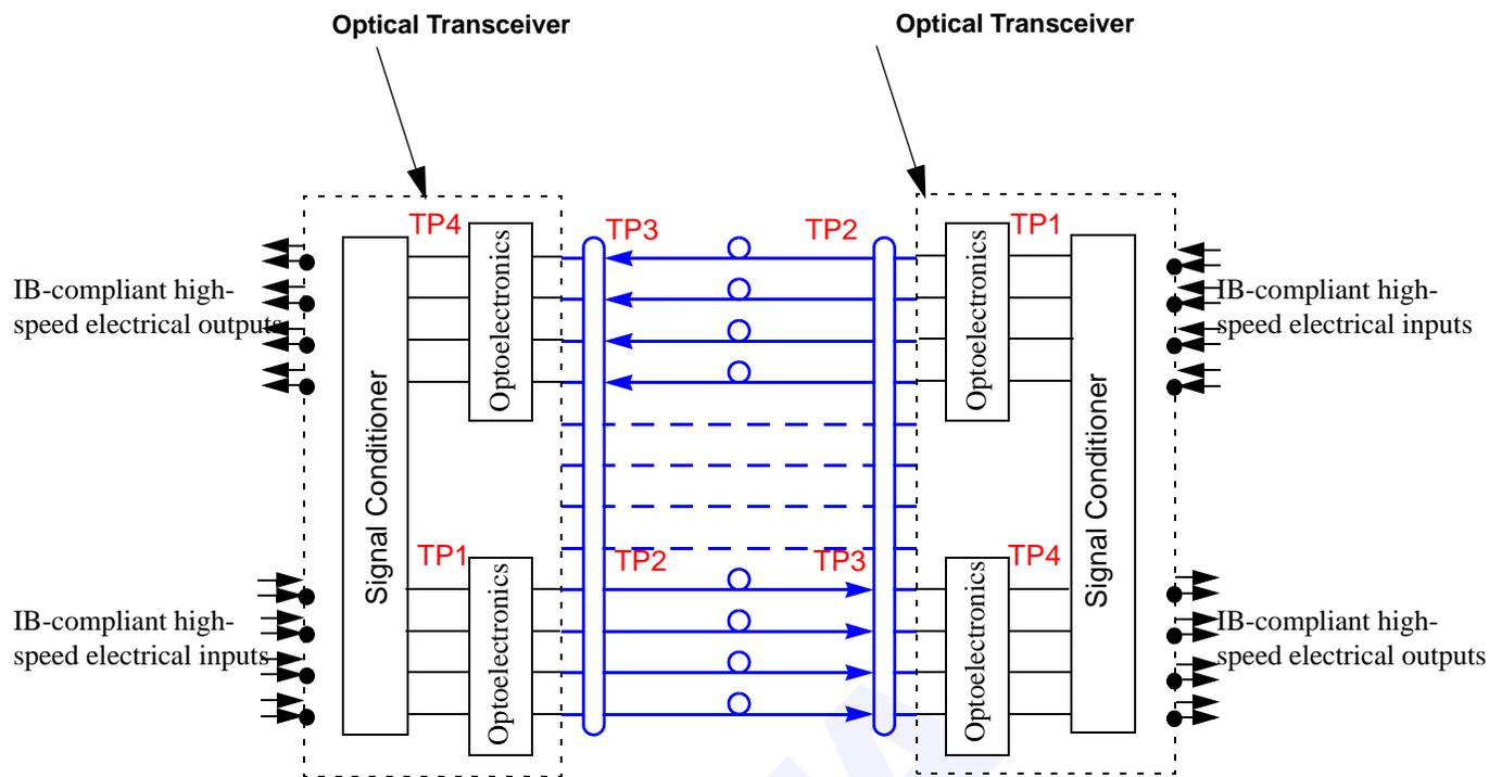
**Figure 88 Recommended 4x-SX & 4x-DDR-SX Optical Link Implementation**
