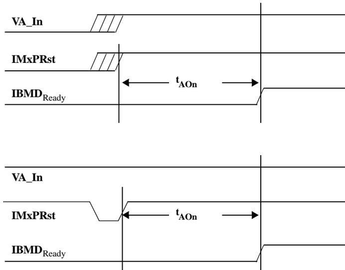
Figure 147 VA\_In Timing Measurements
