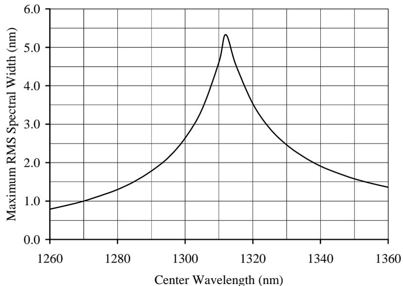
**Figure 76 1x-LX Trade-off between RMS Spectral Width and Center Wavelength**
