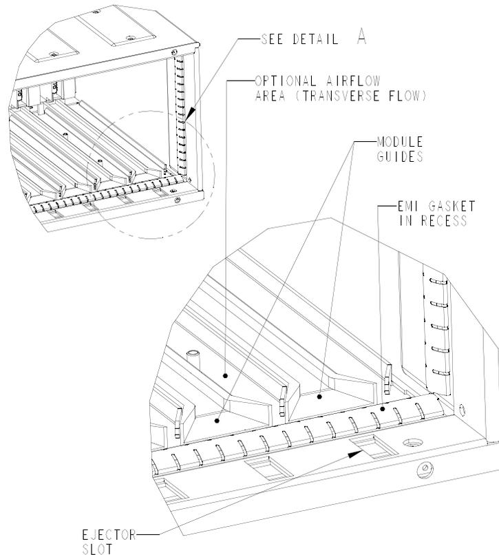
Figure 94 Chassis Slot Detail
