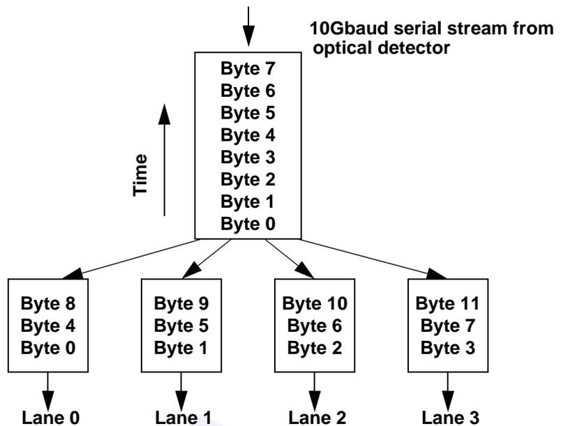
Figure 69 4x LX receiver de-serialization
