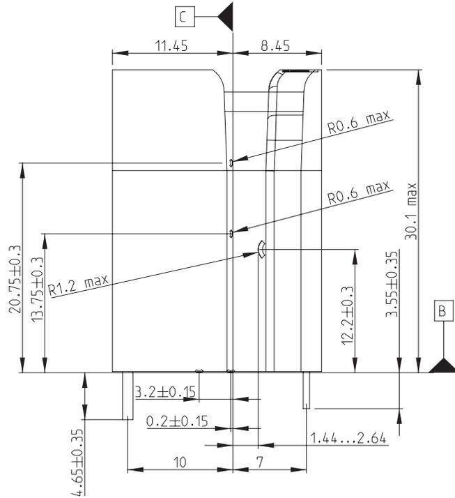
Figure 138 Contact resting locations on board
