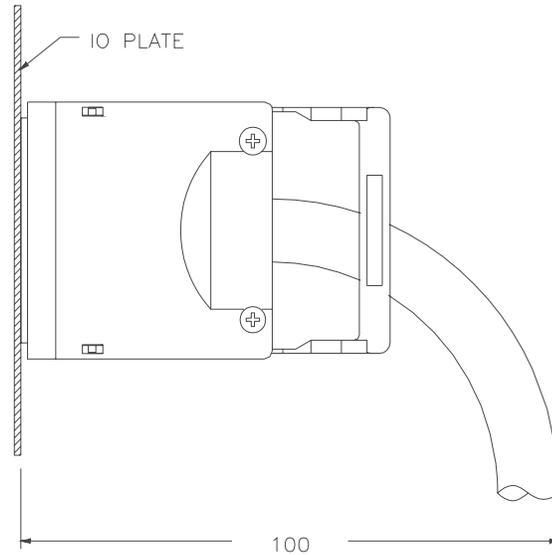
**Figure 59 Cable assembly bend radius**
