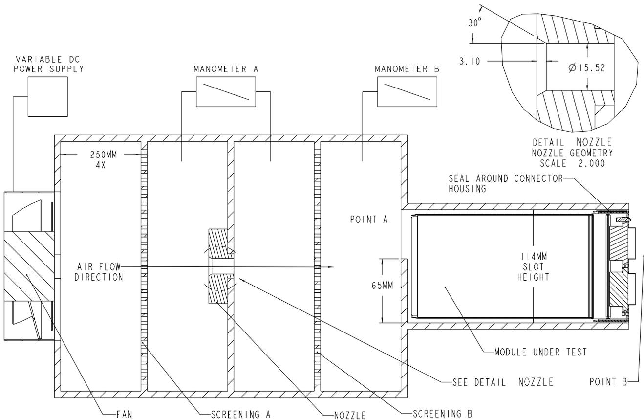
**Figure 192 Schematic of pressure drop test fixture**
