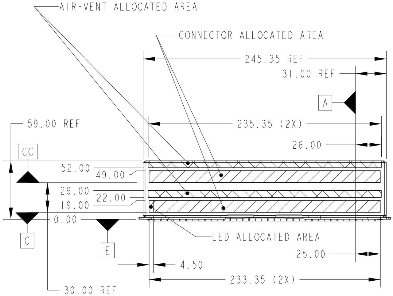
**Figure 111 Tall Wide Critical Dimensions - Detail C**
