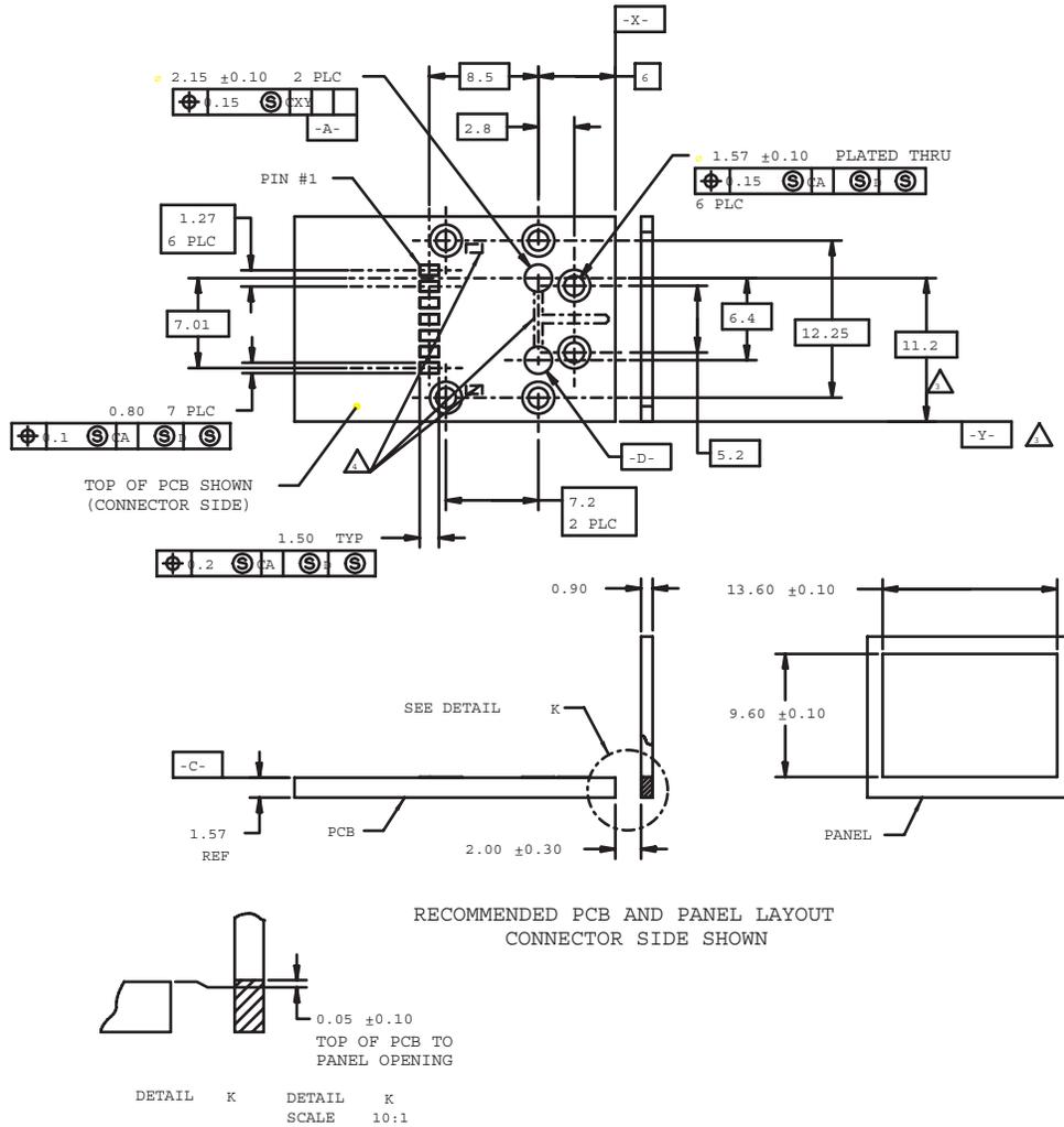
Figure 46 1x cable board connector footprint (top view) and panel layout
