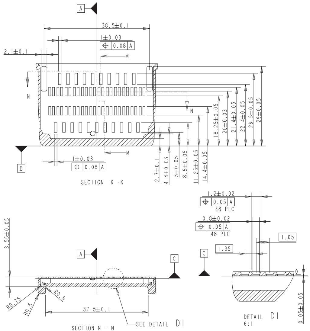
Figure 133 Paddle guard contact window detail, board primary side
