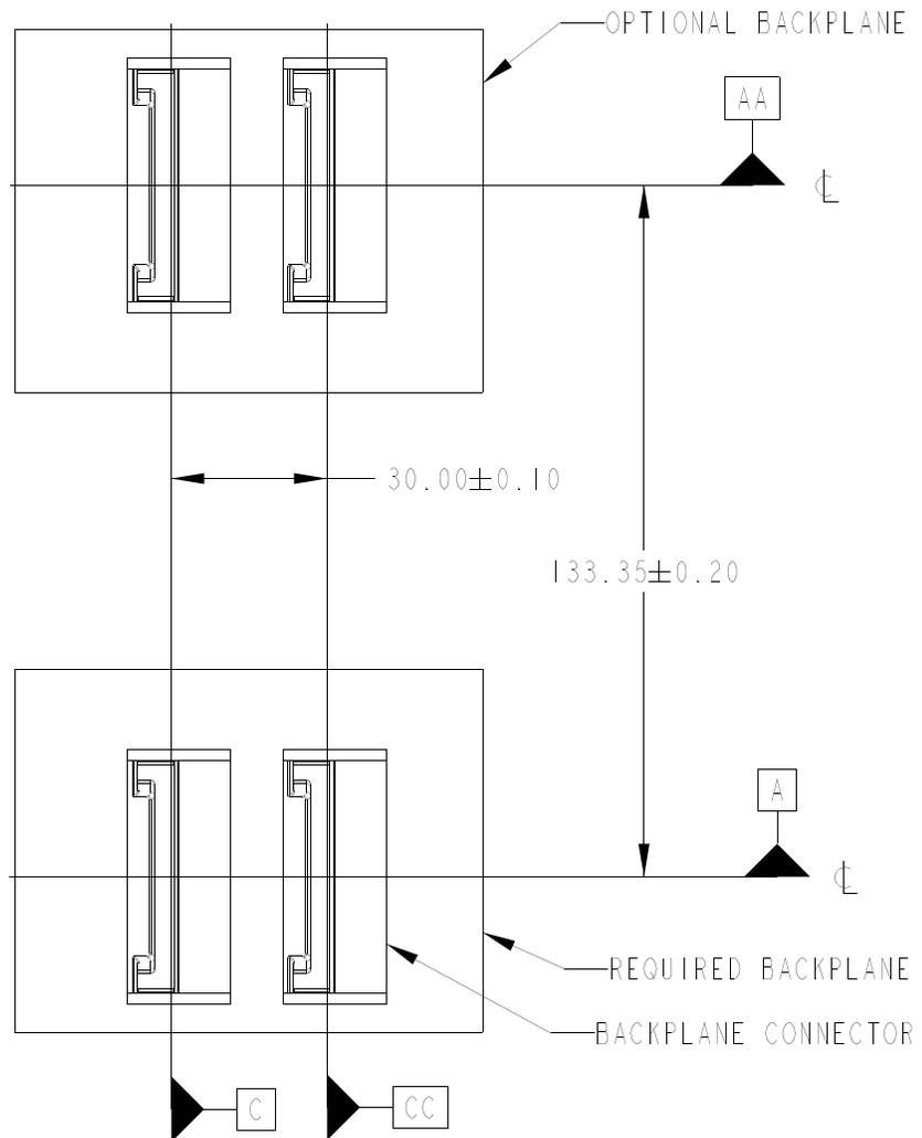
**Figure 121 Backplane Connector Spacing**
