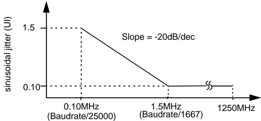
Figure 75 Jitter Tolerance Mask
