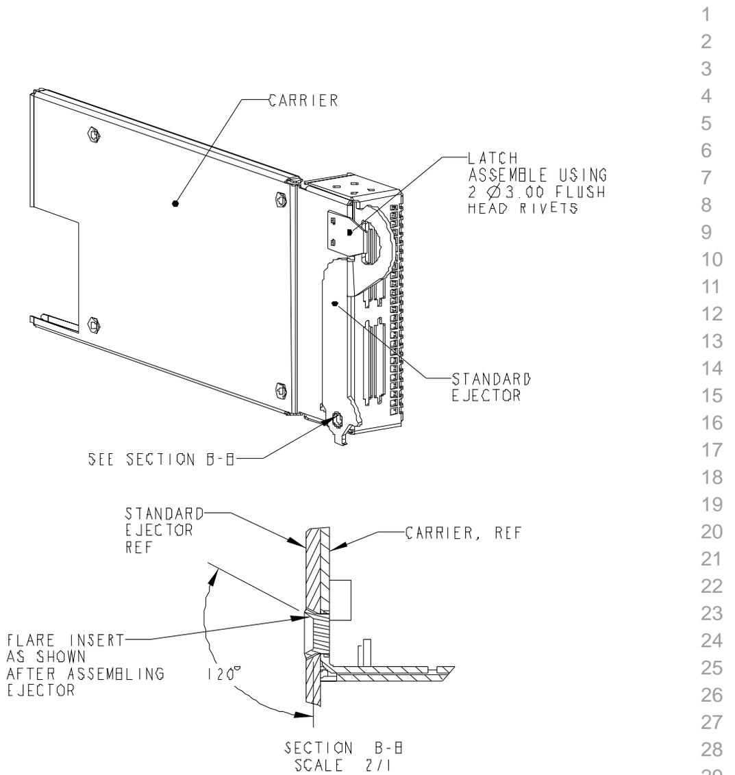
**Figure 188 Example IB Carrier Assembly Details**
