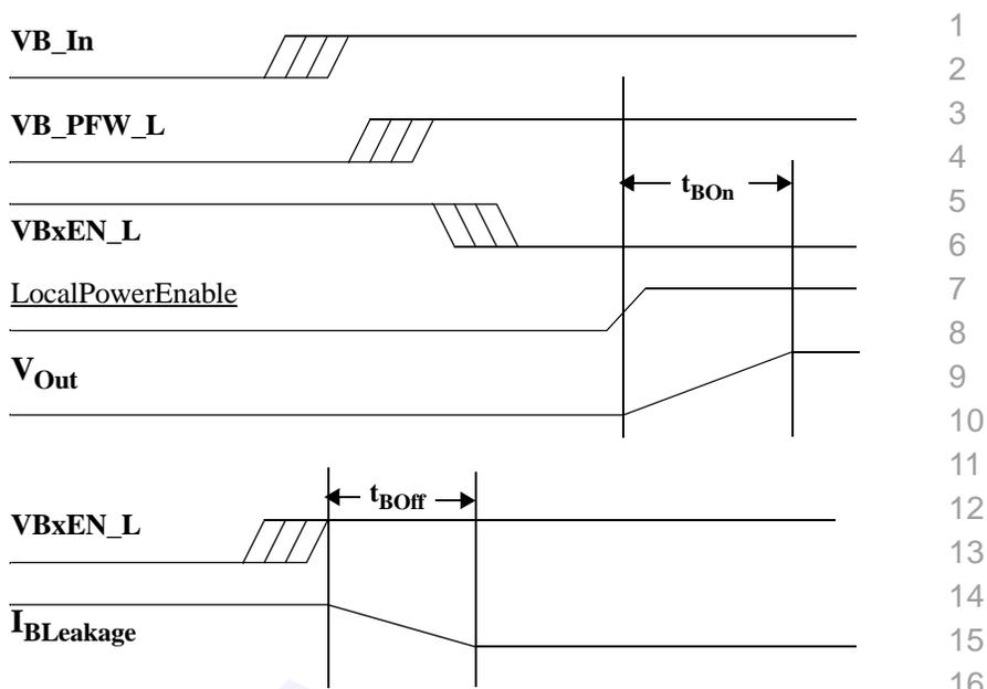
Figure 146 VBxEn\_L Timing Measurements
