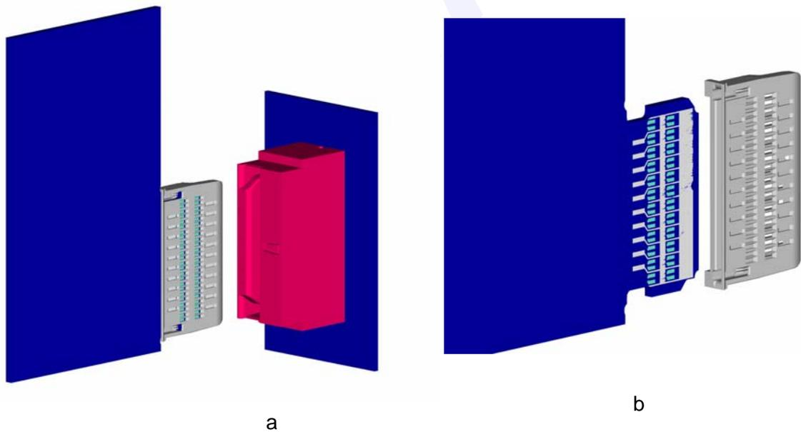
**Figure 128 Backplane connector and board paddle (a), paddle guard assembly (b)**
