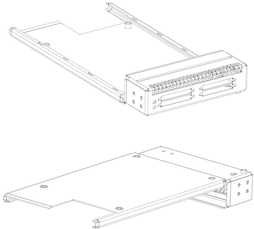
**Figure 184 Example IB Module Carrier**
