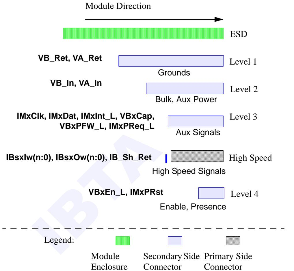
**Figure 156 Module Removal Contact Sequence**
