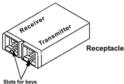
**Figure 83 4x-LX Optical Receptacle orientation**
