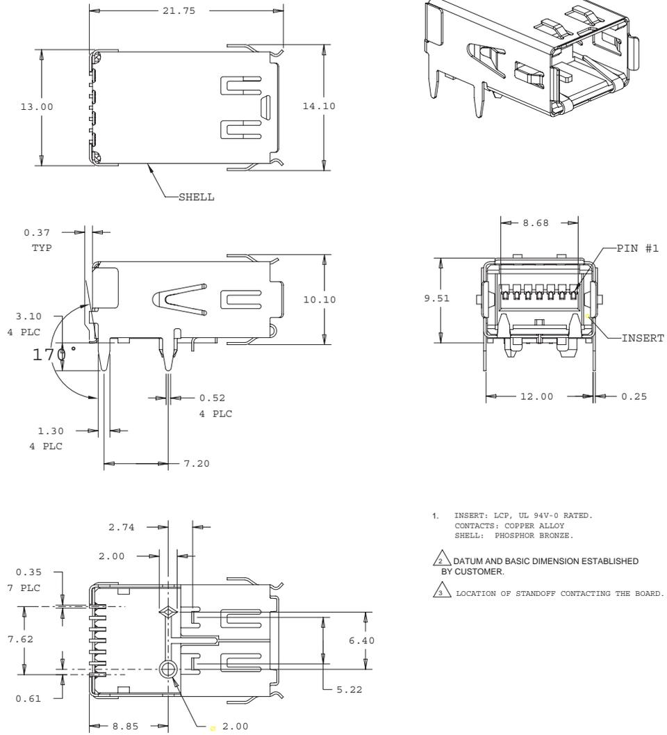
Figure 44 1x cable board connector
