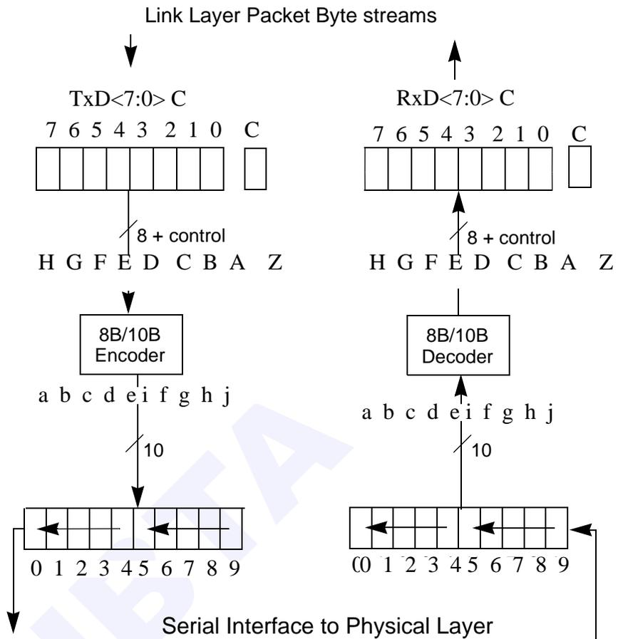
Figure 10 Transmit & Receive Data Ordering
