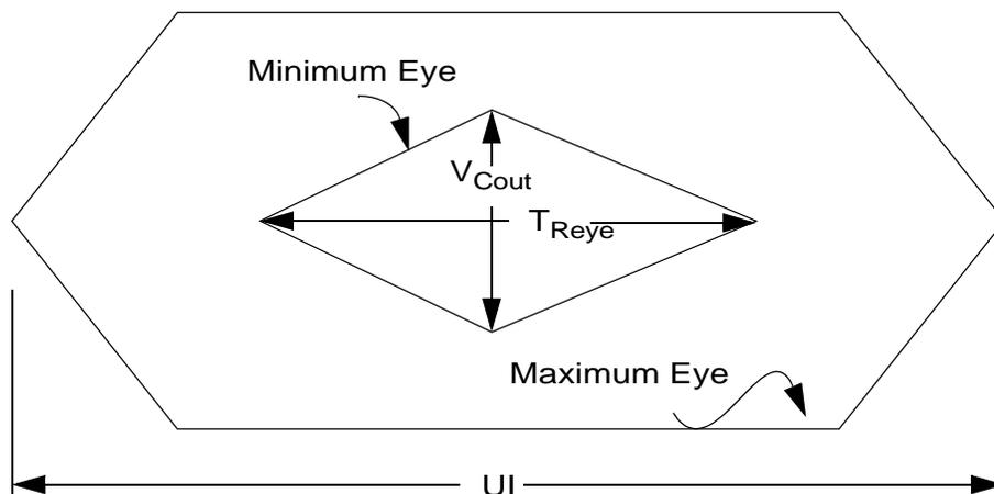
Figure 60 Eye Opening at receiving board connector pins (differential)
