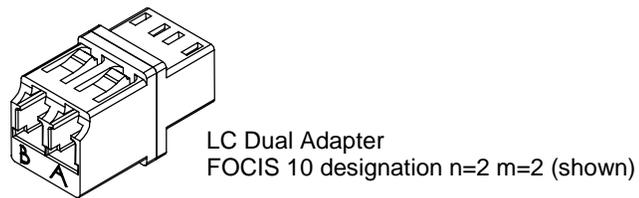
**Figure 79 Dual LC Fiber Optic Adapter**
