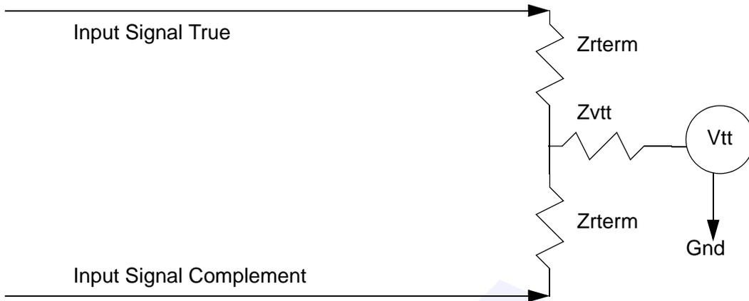
Figure 32 Termination and Signaling
