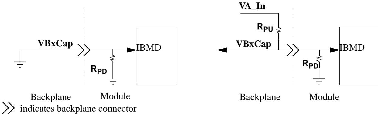
Figure 144 VBxCap Termination - 50W IB Module
