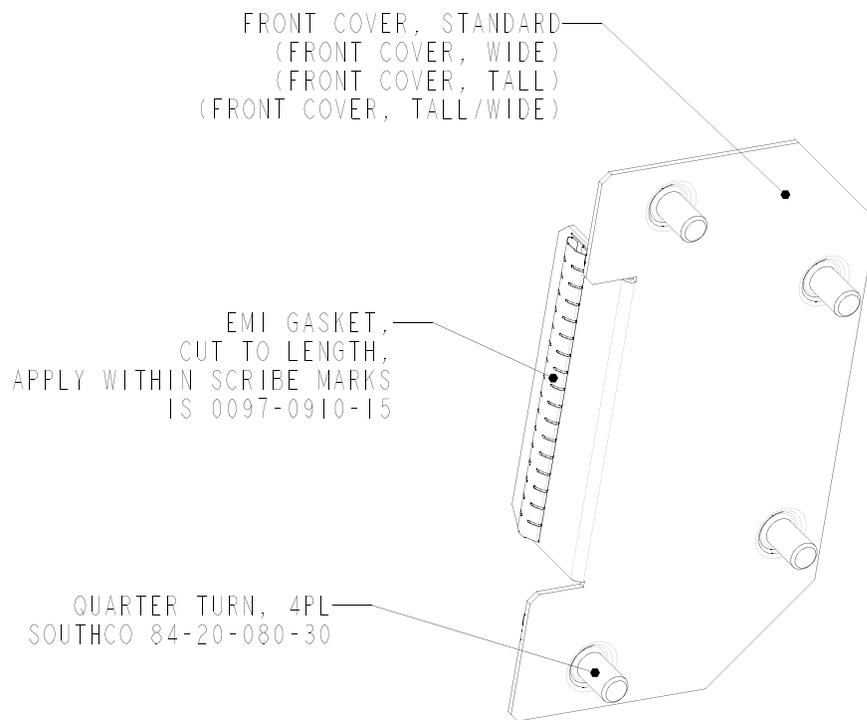
**Figure 212 Front Cover Assembly - Standard; Wide; Tall; Tall/Wide**
