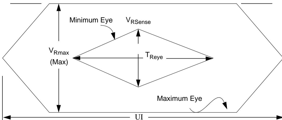
**Figure 31 Eye Opening at receiver (Differential)**
