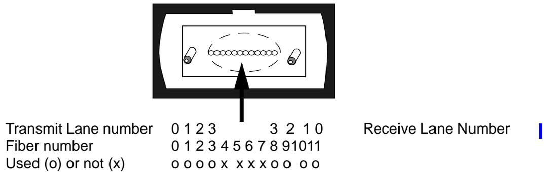
**Figure 82 4x-SX Optical Receptacle orientation looking into the Transceiver**
