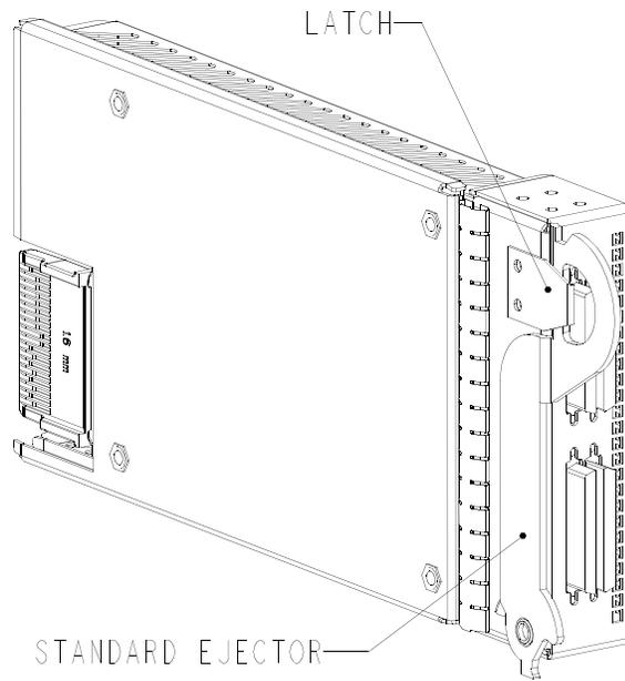
Figure 113 Standard Module With Ejector and Latch
