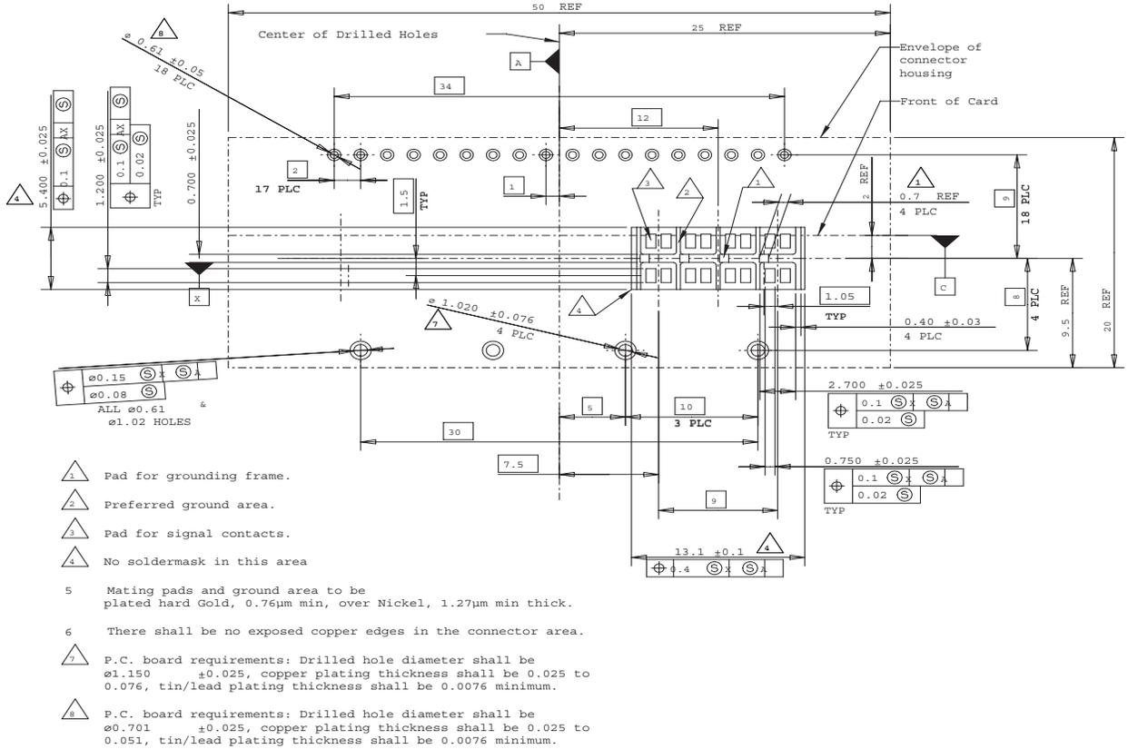
Figure 141 Backplane connector footprint for 1x/4x port
