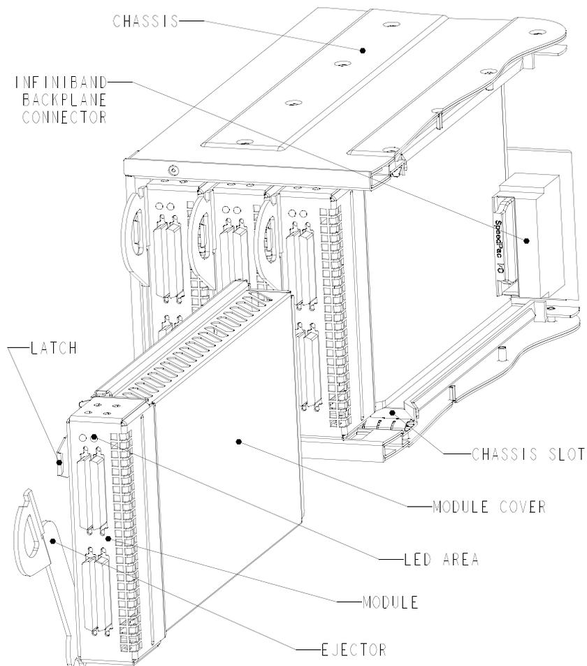
**Figure 92 Standard Module, 3U Chassis Slots**
