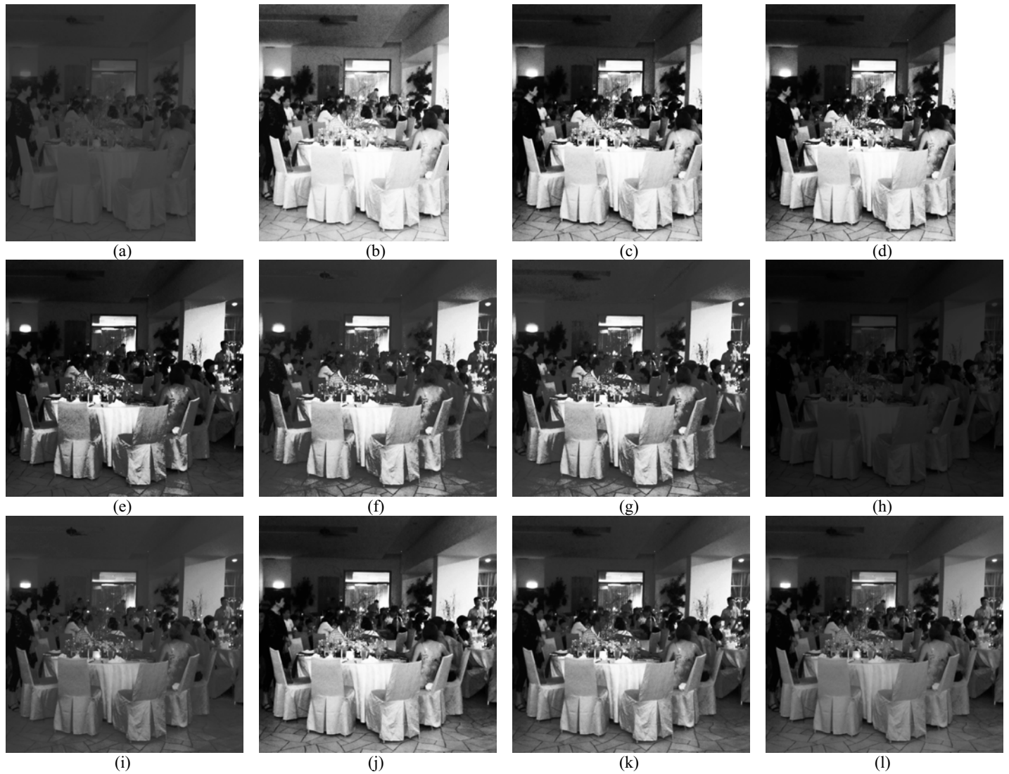
Fig. 4. Image of 'Dinner'. (a) Original image, (b) HE-ed image, (c) BBHE-ed image, (d) DSIHE-ed image, (e) MMBEBHE-ed image, (f) RMSHE-ed image, (g) RSIHE-de image, (h) BPDHE-ed image, (i) RWSHE-M-ed image, (j) BHEPL-ed image, (k) DQHEPL-ed image, (l) BHEPL-D-ed image.
