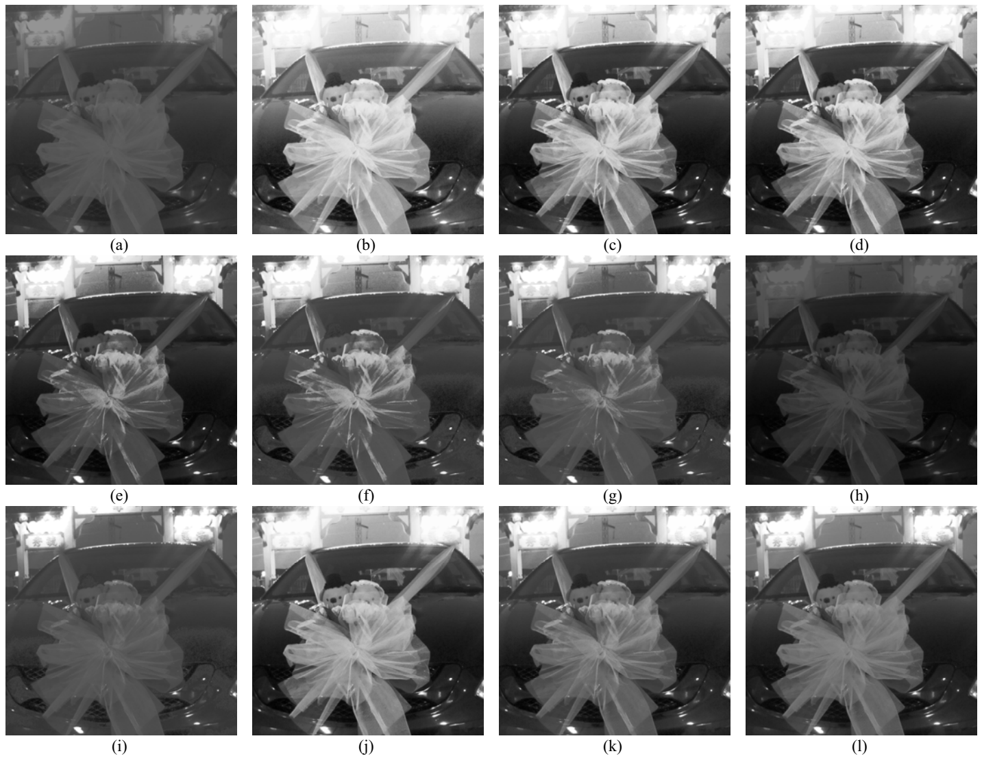
Fig. 5. Image of ‘Car’. (a) Original image, (b) HE-ed image, (c) BBHE-ed image, (d) DSIHE-ed image, (e) MMBEBHE-ed image, (f) RMSHE-ed image, (g)RSIHE-ed image, (h) BPDHE-ed image, (i) RWSHE-M-ed image, (j) BHEPL-ed image, (k)DQHEPL-ed image, (l) BHEPL-D-ed image.
