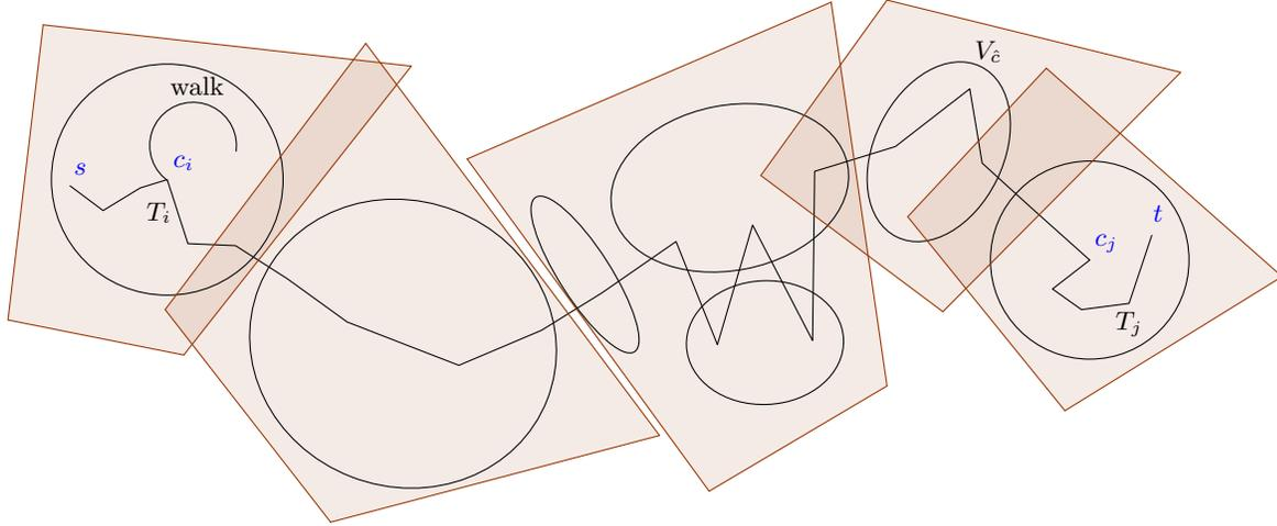
**Figure 2: Trail Routing Example:** from source  $s$  to center  $c_i$  on tree  $T_i$ , on walk to collect routing information, on trail to  $c_j$  using the internal scheme within cells and gates between cells, and then on  $T_j$  to  $t$ .
