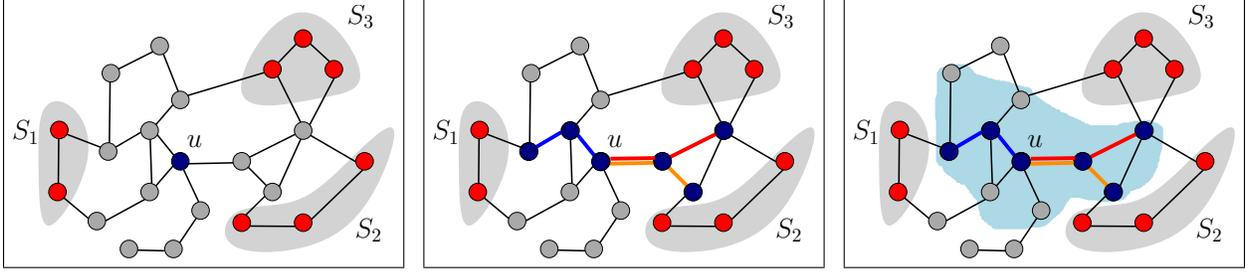
Figure 4.1: An iteration of the algorithm. On the left, there are three supernodes  $S_1, S_2, S_3$  neighboring the current component with  $u$  as a root. In the middle, we have a tree  $T_4$  comprised of three shortest paths from  $u$ . On the right, the new supernode  $S_4$  which is a 1-neighborhood of  $T_4$  (observe that this neighborhood is taken in the connected component containing  $u$ ).
