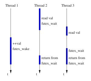
This diagram represents the execution of a program with three threads. Each thread's execution is represented by a vertical line, progressing with time downward. The blue parts are those at which the thread actually has a CPU. If two or more blue lines overlap vertically the threads are executed concurrently.
